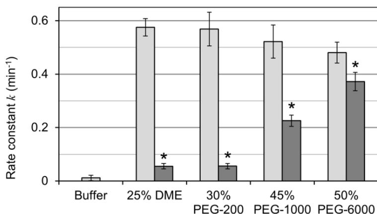
Figure 11. Effect of salt on the rate constant of strand exchange. An asterisk (\*) indicates that salt was added to compensate for the loss of stability caused by a base mismatch. Longer PEG polymers retain more catalytic ability at high salt concentration than shorter PEG/DME.
