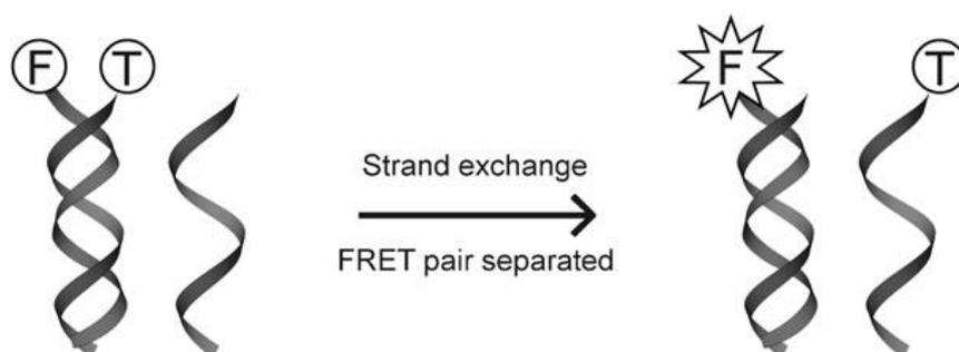
Figure 6. The principle behind FRET-based strand exchange assay, in which recovery of FAM fluorescence is directly proportional to the exchange yield.
