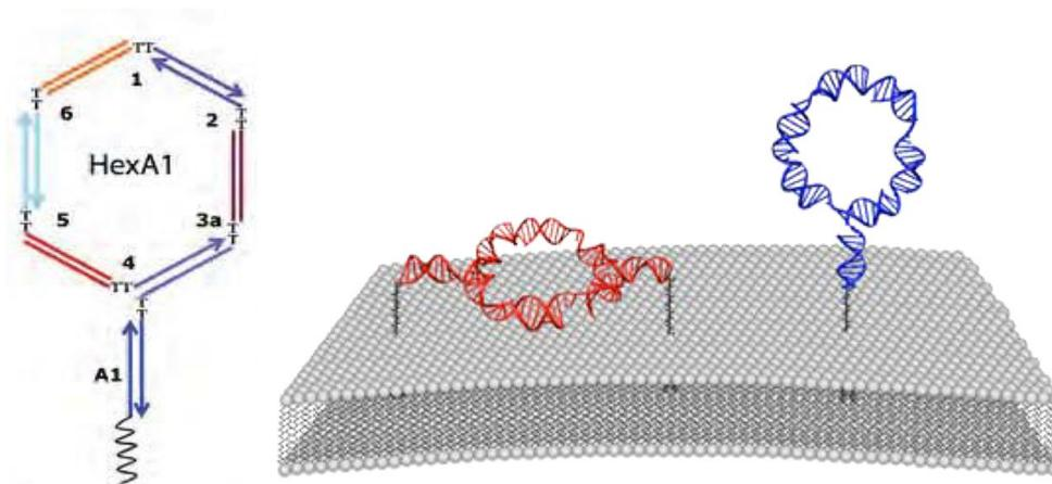
Figure 12. The DNA hexagon is self-assembled from individual DNA strands and anchored to the membrane surface using fatty acid chains. Either protruding (HexA1) or flat (HexA2) orientation is obtained by using one or two anchors.
