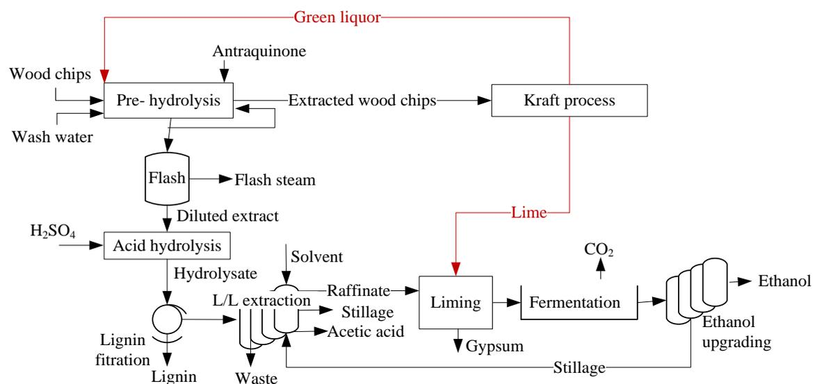
Figure 6 Near-neutral hemicellulose extraction process.
