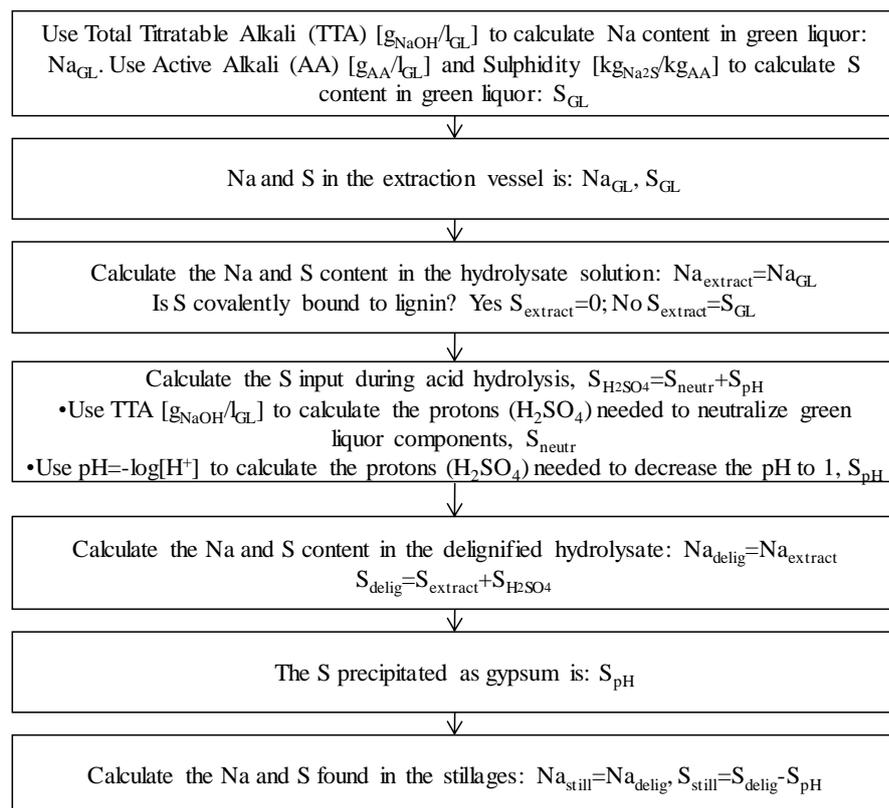
Figure 9 Method to develop Na/S balances.
