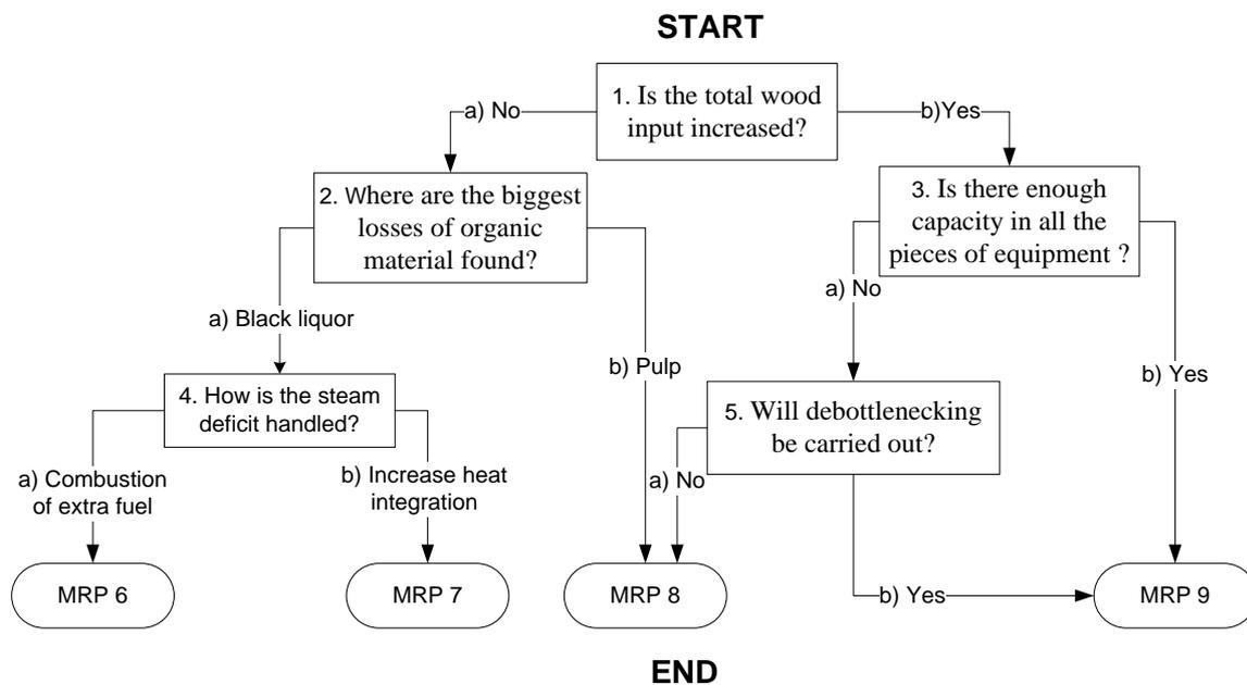
Figure 19 Quick reference guide flowchart. MRP: minimum requirement for profitability.
