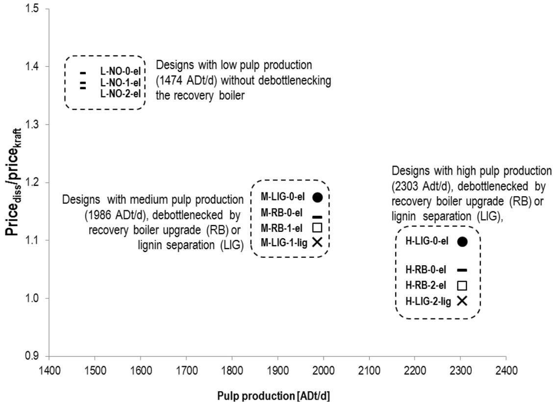
Figure 14 Ratio between dissolving and kraft pulp prices that makes the annual earnings equal for both the kraft and the dissolving pulp mill. To calculate the revenues from lignin sales, a lignin price of 35 €/MWh-lig was used (valued as heavy fuel oil).
