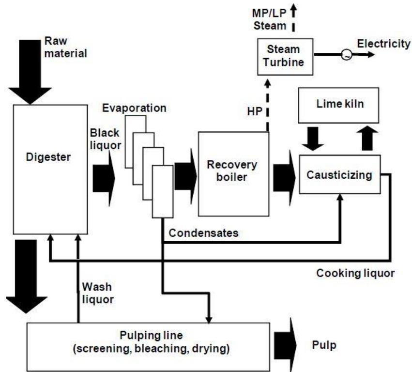
Figure 2 Block flow diagram of the kraft pulping process. Image reproduced from Fornell, 2012.
