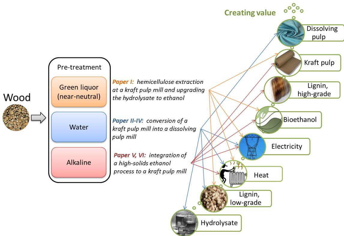
Figure 3 Types of pretreatment methods used and products and by-products produced in the studied biorefineries.
