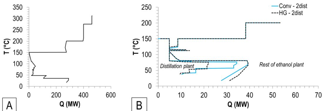
Figure 16 Potential for heat integration. 19A, Left: GCC of the pulp mill. 19B, Right: Foreground/background analyses of the distillation plant and the remainder of the ethanol plant.
