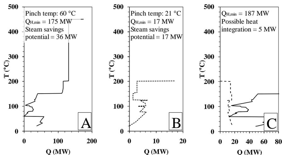
Figure 10 Grand composite curves. 13A, Left: Pulp mill. 13B, Middle: Bioethanol plant. 13C, Right: Foreground-background analysis.
