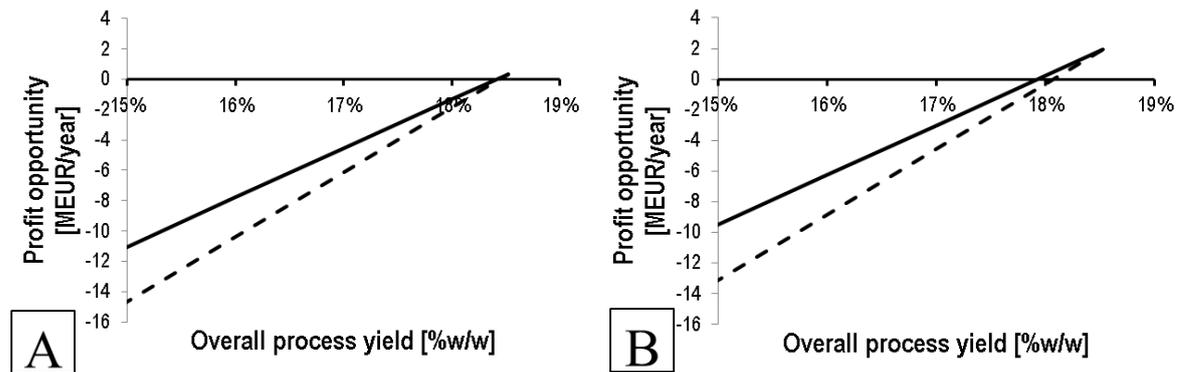
Figure 18 Profit opportunity for the high-gravity process. The solid and dashed lines are calculated with ethanol prices of 500 and 650 €/m<sup>3</sup>, respectively. 15A, Left: stillage to effluent treatment. 15B, Right: stillage to PMEPE.
