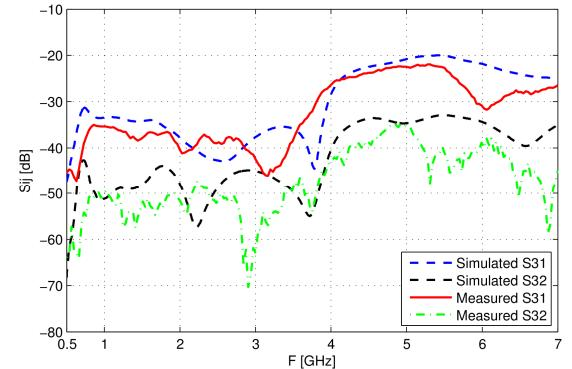
Figure 8. Simulated and measured mutual coupling between antenna 1 (LTE) and 3 (V2X) and between antenna 2 (LTE) and 3 (V2X).
