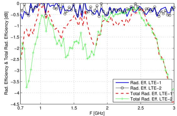
Figure 9. Measured radiation efficiency and total radiation efficiency for the LTE antennas.
