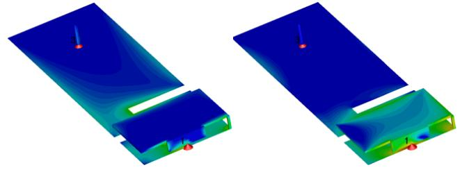
Figure 2. Current distribution at 698 MHz (left) and 2690 MHz (right).
