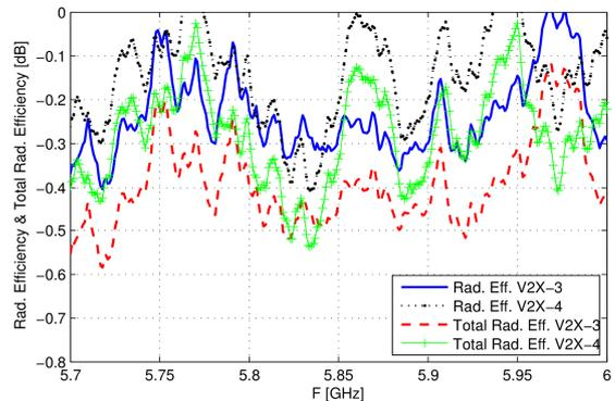
Figure 10. Measured radiation efficiency and total radiation efficiency for the V2X antennas.
