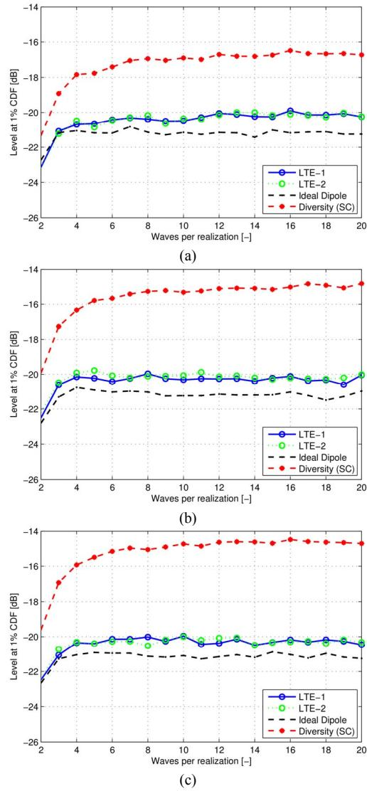
Figure 13. Received power at 1% CDF-level as a function of linearly polarized incident waves for LTE at three different frequencies. (a) 830 MHz, (b) 1940 MHz, (c) 2590 MHz. Diversity selection combining is also shown in the graph.
