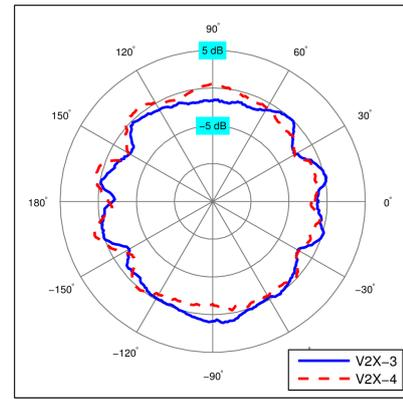
Figure 12. Measured radiation pattern (total gain) for V2X in the azimuth plane.
