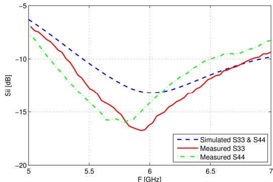
Figure 6. Simulated and measured return loss of the antenna module for V2X antennas.
