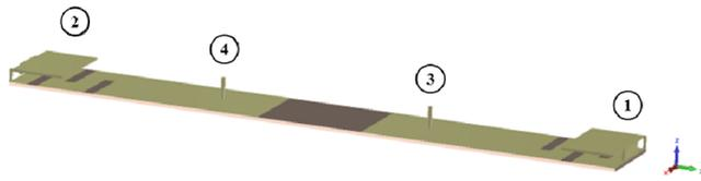
Figure 3. Antenna module for LTE and V2X communications.
