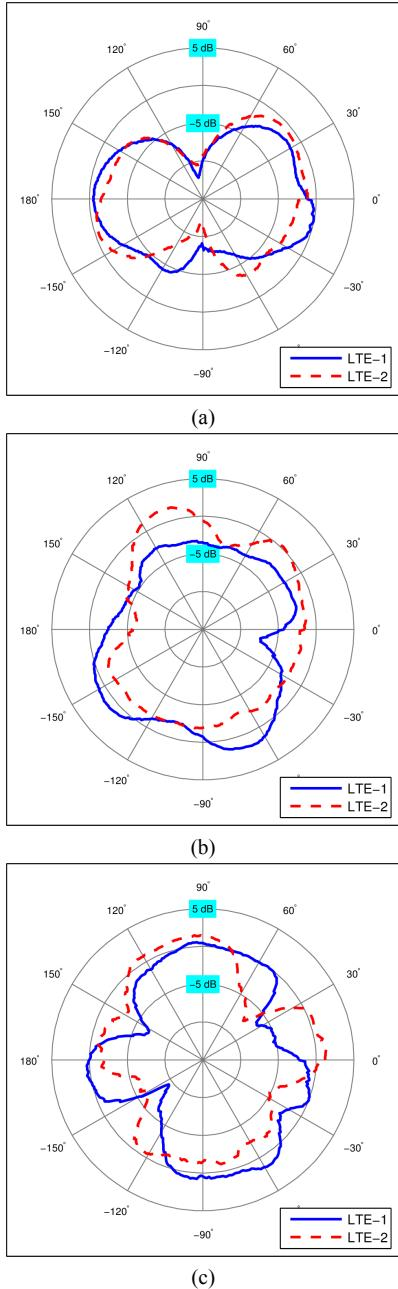
Figure 11. Measured radiation patterns (total gain) for LTE in the azimuth plane. (a) 830 MHz, (b) 1940 MHz, (c) 2590 MHz.
