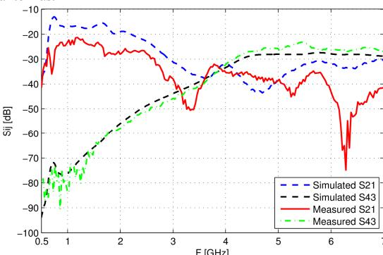
Figure 7. Simulated and measured mutual coupling between antenna 1 and 2 (LTE antennas) and between antenna 3 and 4 (V2X antennas).
