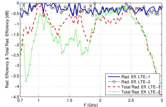
Figure 9. Measured radiation efficiency and total radiation efficiency for the LTE antennas.
