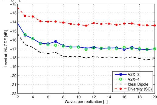
Figure 14. Received power at 1% CDF-level as a function of vertical polarized incident waves for V2X, i.e., 5.9 GHz. Diversity selection combining is also shown in the graph.
