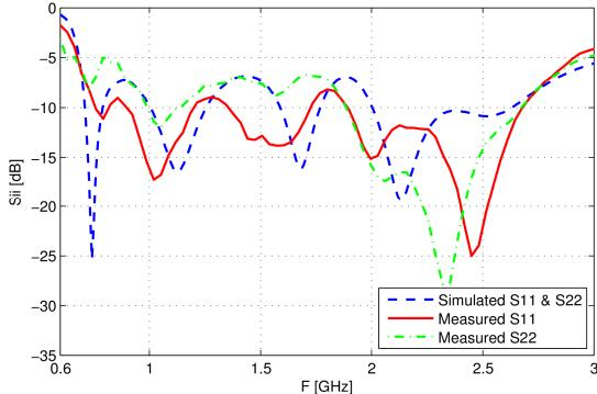
Figure 5. Simulated and measured return loss of the antenna module for LTE antennas.
