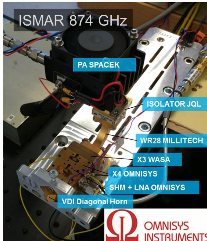
Figure 4. Prototype setup for the ISMAR 874 GHz front-end receiver MMIC system.
