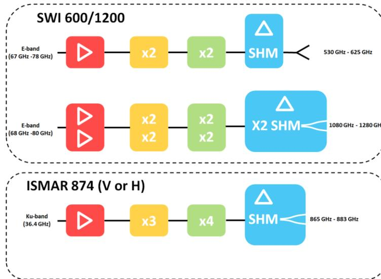
Figure 2. Schematic of the SWI 600 GHz and 1200 GHz receiver channels and ISMAR 874 GHz V/H channels.
