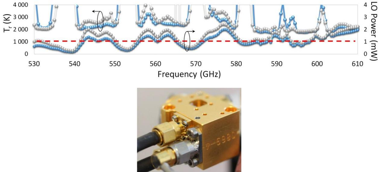
Figure 5. Measured performance (top) and photograph (bot), of the SWI 530-625 GHz receiver front-end prototype.
