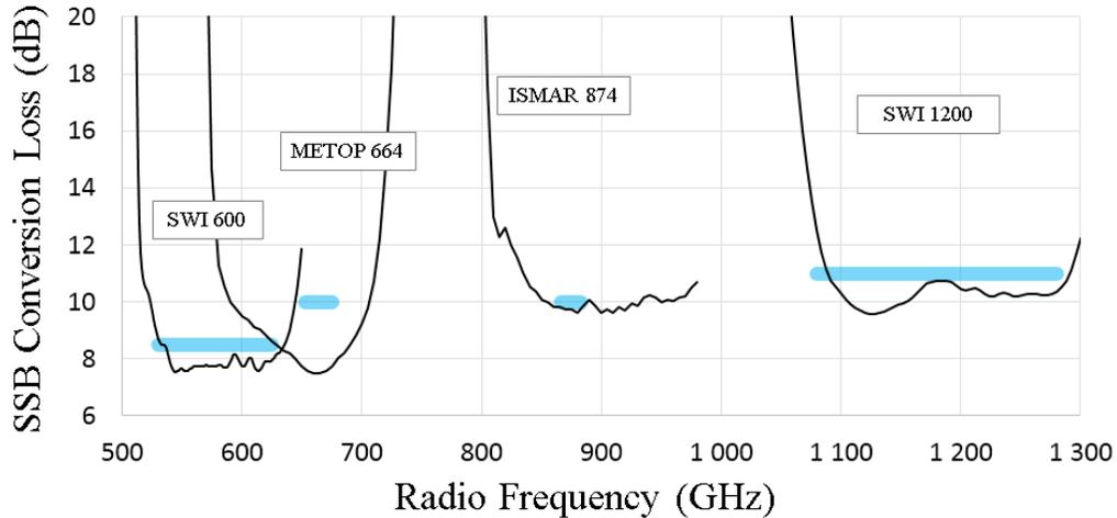
Figure 3. Simulated mixer performance based on full 3D-EM models for four different Omnisys TMIC designs. The simulations were performed at fixed LO powers ranging from 1.2 mW to 1.8 mW.
