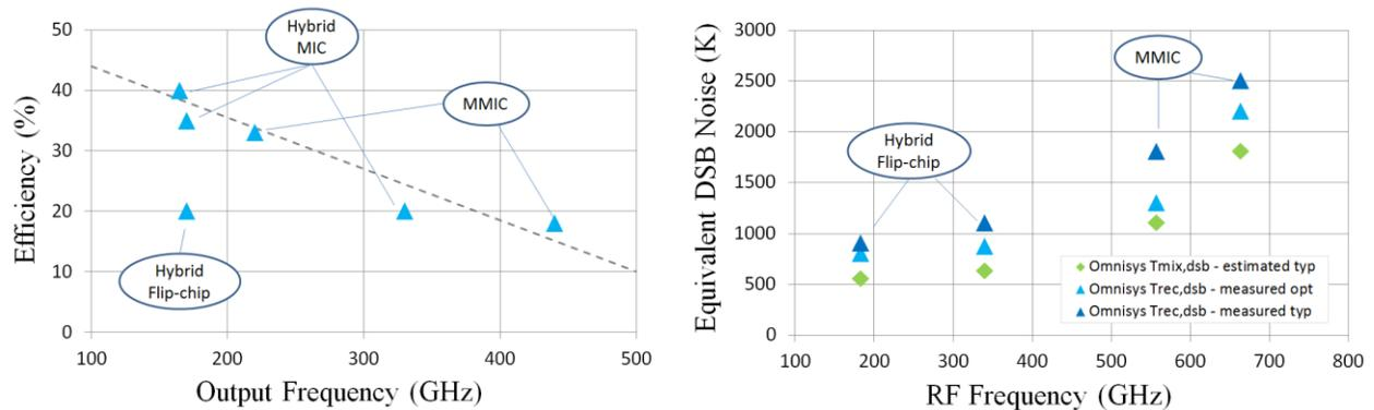
Figure 6. Short summary of Omnisys receiver systems showing measured receiver noise temperature (right) and x2 multiplier efficiency (left).
