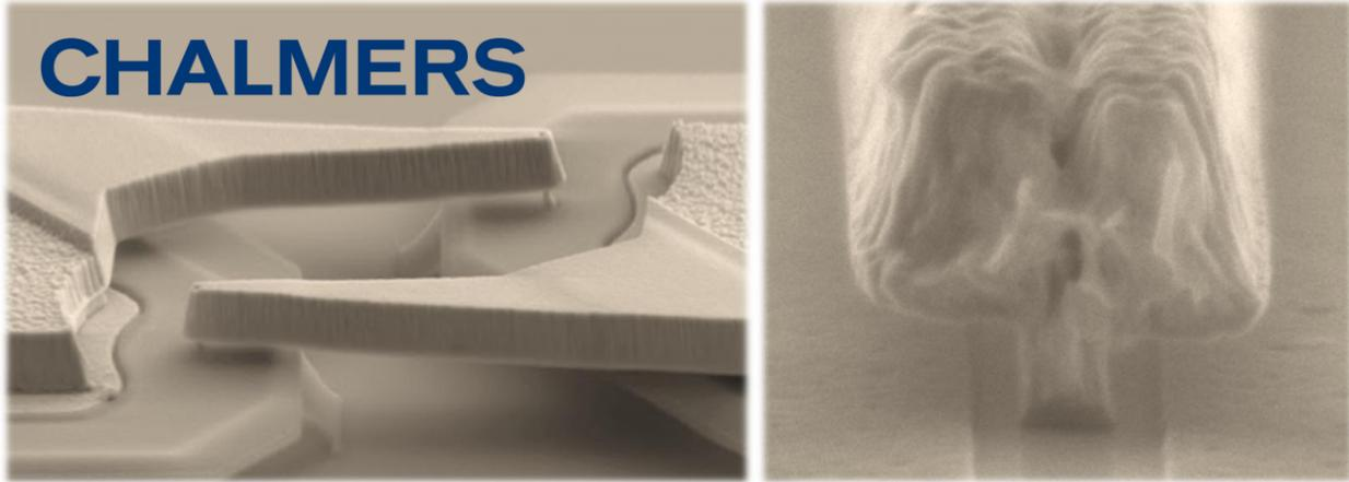
Figure 1. SEM of a 1.2 THz antiparallel Schottky diode structure and cryogenic InP HEMT transistor from CHALMERS. The anode size and gate length of the devices are  $\sim 0.1 \mu\text{m}^2$  and  $\sim 50 \text{ nm}$  respectively.
