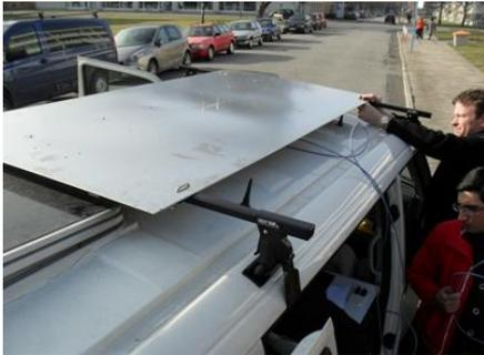
a) Metal sheet under car roof
