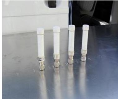
b) Ghost antennas in front and behind the measurement antennas
