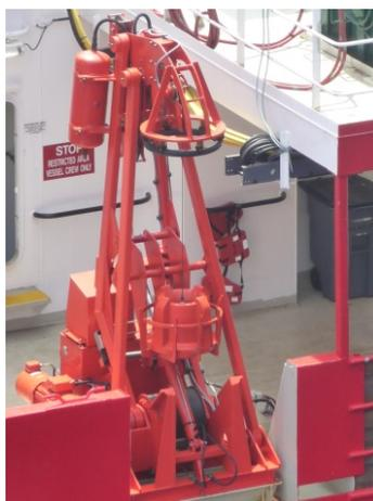
Figure 6.5. Light Taut Wire Crane (CC-BY-SA License by BoH)
