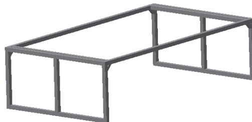
**Figure 4.7. Principle sketch of the fixture to be used during operations with foundations.**
