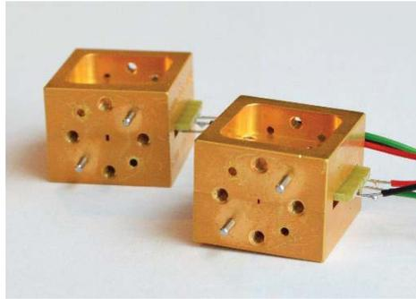
Fig. 5.8. Fabricated WR05 and WR03 amplifier modules [D].
