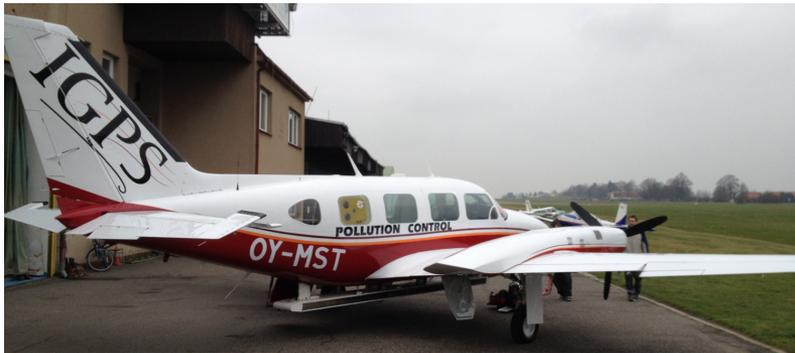
Figure 7.1: The Navajo Piper airplane with certified, permanent installation of the airborne IGPS system (courtesy of Tue Friis-Hansen).
