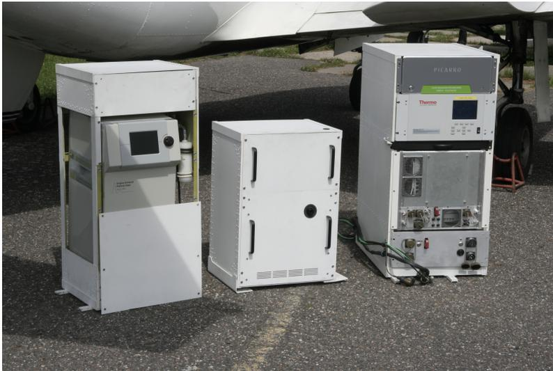
Figure 7.3: The gas rack (right) contains instrumentation for measurements of  $\text{CO}_2$ ,  $\text{SO}_2$  and  $\text{NO}_x$  as well as a buffer battery and the main computer. The particle rack (left) includes instrumentation to assess the exhaust aerosol's particle size distribution.  $\text{SO}_2$  and  $\text{NO}_2$  is also analyzed using the spectrometers in the optics rack (middle).
