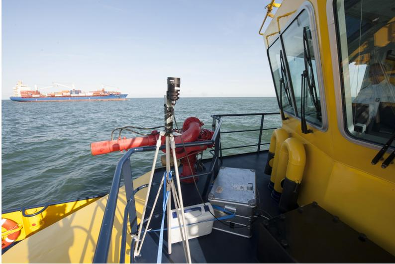
Figure 6.1: Upward looking optical system. Here an upward looking telescope is connected an optical fiber which transmits light into a UV/visible spectrometer measuring wavelengths between 300 to 324 nm (courtesy of Jacob Balzani Lööv) .
