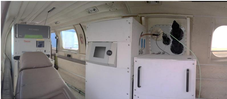
Figure 7.5: One window probe plate and three instrument racks for ship emission measurements in a Navajo Piper airplane.
