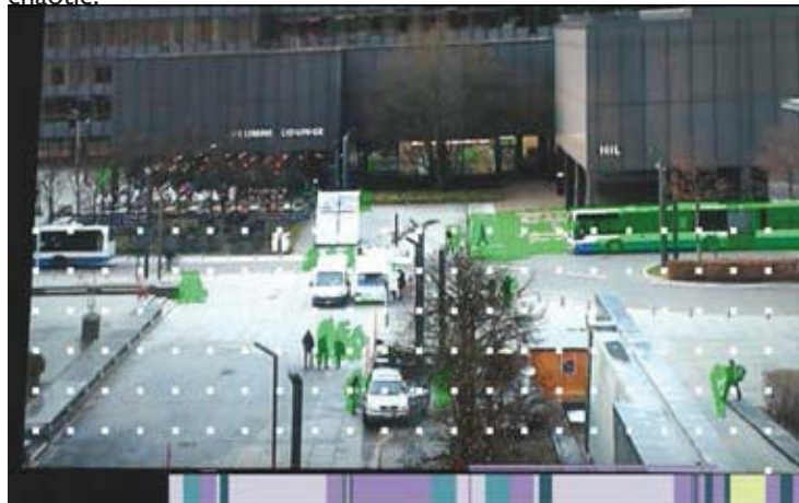
Figure 5. Testing and demonstrating the capacity to predict. The algorithm was shown the video twice, and the second time it was able to use the first as prediction. Prediction is displayed in green.
