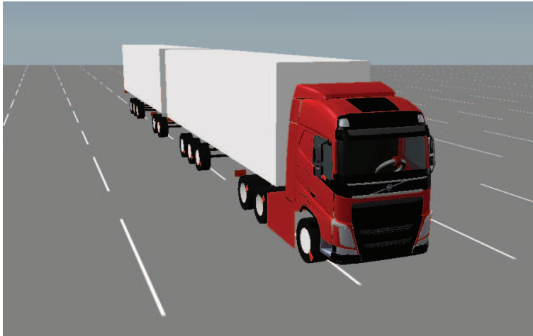
Figure 3: A long vehicle combination with eleven axles and 26 tyres.
