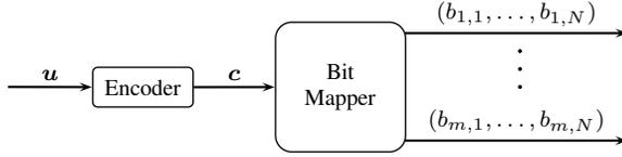
Fig. 3. Illustration of the Bit Mapper.
