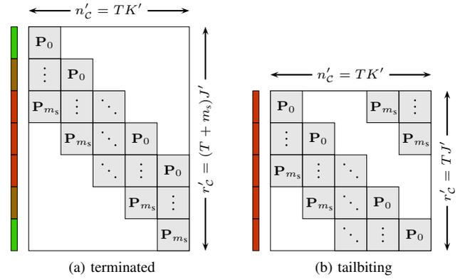
Fig. 4. Base matrices  $\mathbf{P}$  for protograph-based SC-LDPC codes.
