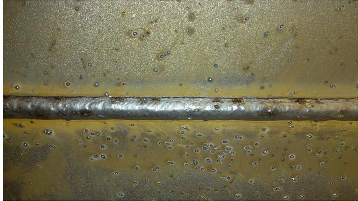
Figure 5.2: Changes in reflectivity, and emissivity, are apparent for this welded steel specimen.
