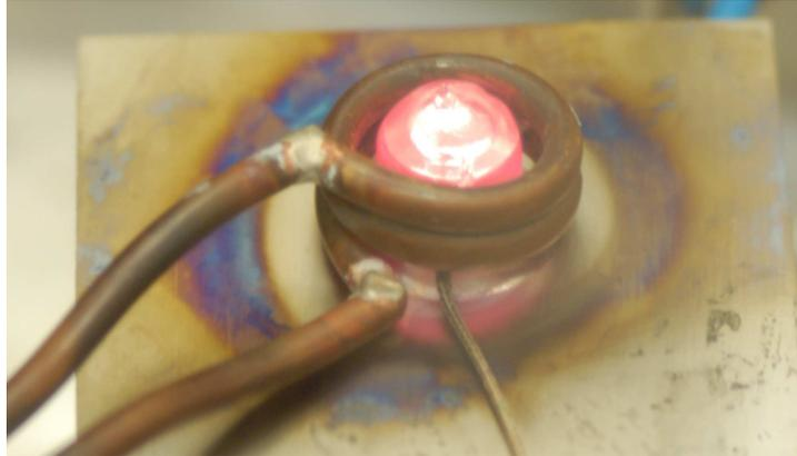
Figure 6.10: Induction heated titanium specimen. Oxide visible as bluish taint on base plate.
