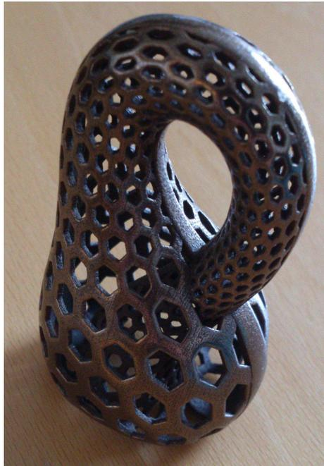
Figure 1.2: Klein bottle manufactured using a powder bed process.
