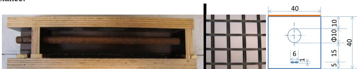
Figure 1 Image of the casting mould (left), the carbon fiber mesh anode (middle) and the dimension of specimen (right).
