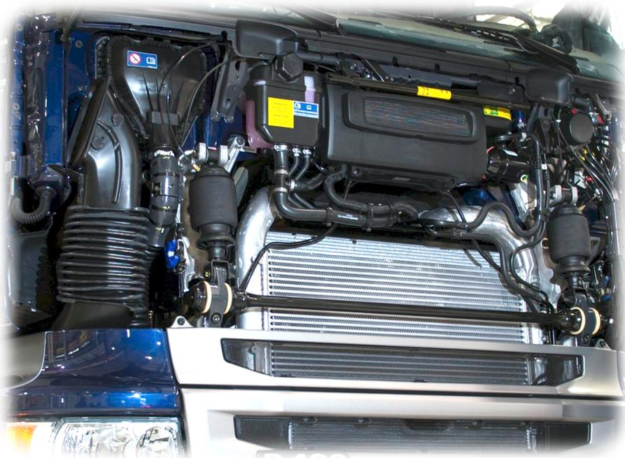
Figure 1.2: *The underhood of modern vehicles can be tightly packed with components. Designing efficient ducts that connect the different components in this tightly packed compartment is not an easy task. Photo courtesy of Scania.*
