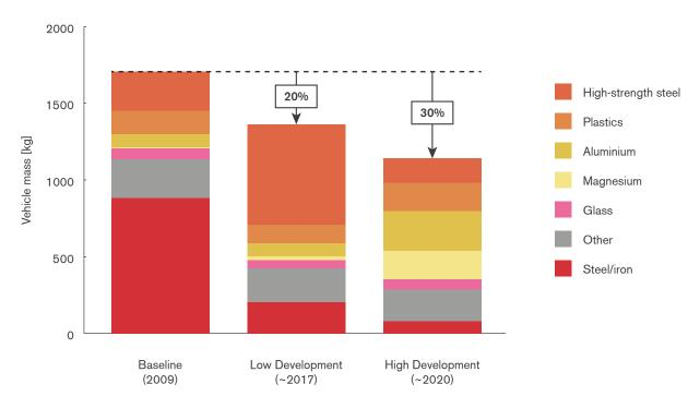
**Figure 7.4.** The mass by material of the Lotus baseline and mass-reduced car designs. Low and High Development illustrate concepts available for model years 2017 and 2020 commercial deployment<sup>18</sup>.
