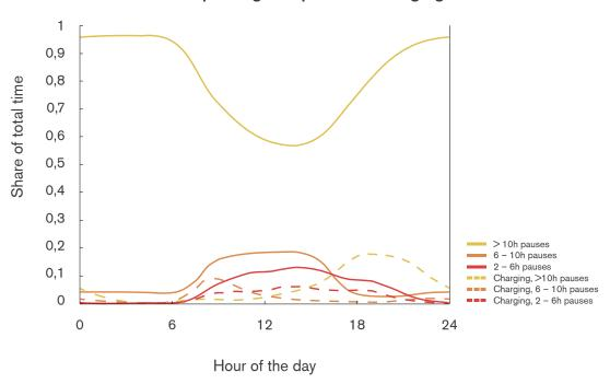
**Figure 9.2** The distribution in time for parking of different lengths and potential charging during these pauses. Assumed: PHEVs with 2 kW charging immediately after parking which continue until battery is full (10 kWh) or pause ends. Energy use 0.2 kWh/km in Charge Depletion mode.<sup>4</sup>
