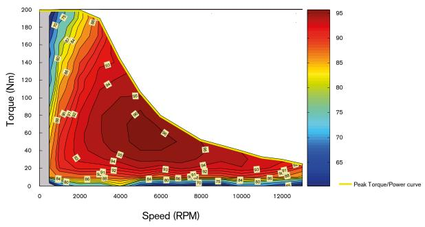
Figure 5.4 2010 Toyota Prius motor efficiency contours.3
