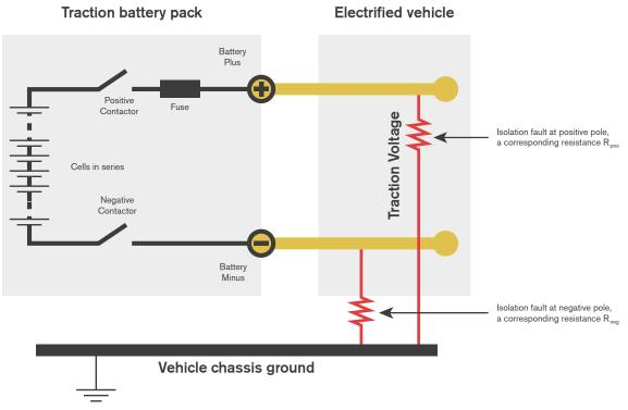
**Figur 4.5** Principle figure that shows a double insulation fault. This means one insulation fault at the plus and one at the minus pole. They are shown as two resistances, Rpos and Rneg, connected to ground. This creates a current path between battery plus and battery minus.
