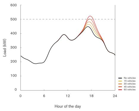
**Figure 9.5** In the status quo case, the vehicles begin charging immediately upon arrival in the residential area. In this example, various numbers of EVs with 2 kW charging are connected in an area served by a 500 kVA transformer. It is seen this strategy can lead to overloading with significant EV penetrations. Note that the capacity for EV penetration will vary greatly from network to network.
