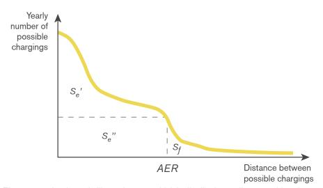
**Figure 10.3** A schematic illustration of a vehicle's distribution of distances driven between charging occasions. The vertical axis is the annual accumulated number of charging occasions followed by a driving above a certain distance before next charging option.
