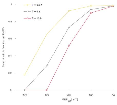
**Figure 10.8** Potential electric drive fraction (EDF) for the car fleet as function of the viability parameter  $MRF_{opt}$  and charging options expressed as pause time T between trips.
