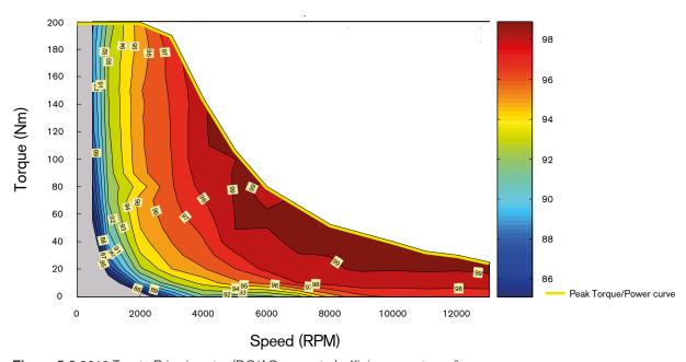
Figure 5.3 2010 Toyota Prius inverter (DC/AC converter) efficiency contours.3
