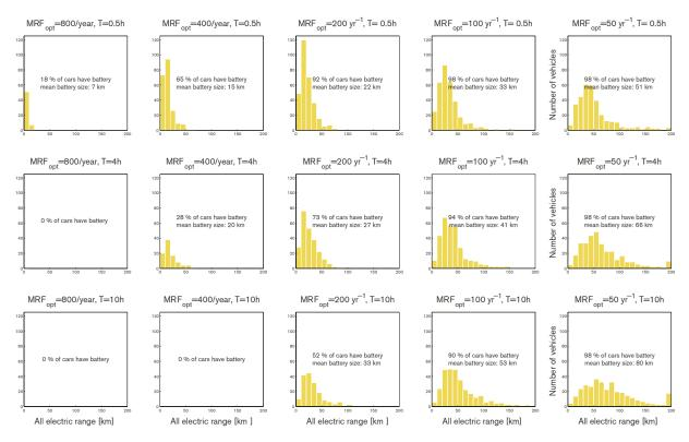
**Figure 10.6** For a total of 326 investigated vehicle movement patterns, the distribution of optimal individual PHEV battery ranges *AER*. From left to right: increasing economic viability, that is, decreasing  $MRF_{opt}$ . From bottom to top: better recharging options, that is, shorter minimum break time T for recharging.
