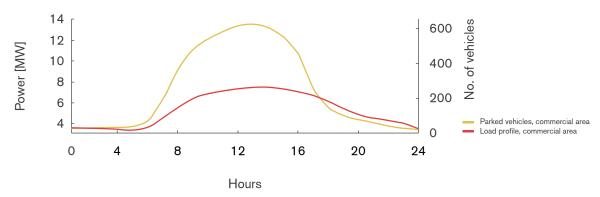
**Figure 9.3** Parked vehicle and load profile comparison for a selected residential and commercial area. Note the correlation between peak loading and vehicle parking in these areas, indicating that uncontrolled charging strategies will increase peak loading constraints.
