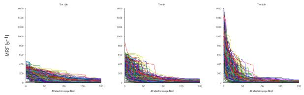
**Figure 10.5** For the individual cars driving pattern, the marginal recharging frequency (MRF) as function of the battery range (AER) and recharging expressed as minimum required break time T for recharging the battery. a) T = 10 hours; b) T = 4 hours; c) T = 0.5 hours.
