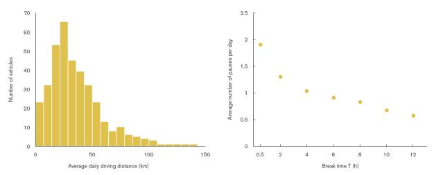
**Figure 10.2** For the logged 212 vehicles, the average daily driving distance and the average number of daily breaks between consecutive trips longer than T hours.<sup>3</sup>.
