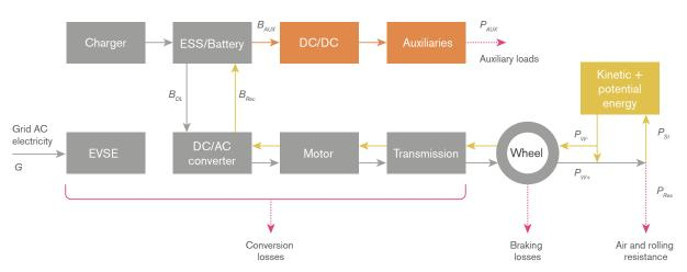
**5.1 The** conversion chain in electric vehicles. Energy is transferred from grid electricity (G), via the battery ( $B_{DL}$  and  $B_{Aux}$ ), to energy at the wheels ( $P_{W+}$ ) and auxiliary equipment ( $P_{Aux}$ ). Part of stored potential and kinetic energy is recovered through the wheels ( $P_{W-}$ ) to the battery ( $B_{Rec}$ ).
