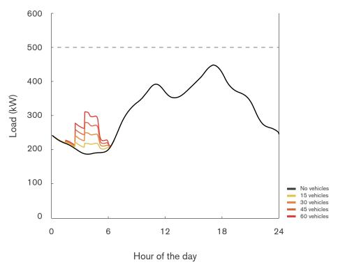
**Figure 9.6** In the hourly pricing scheme, customers will charge their vehicle to meet its transportation energy needs by scheduling to charge during the cheapest available hours. Note that this may cause a localized night-time peak, as is shown for this distribution network. However, if there is system wide adoption of electric vehicles, the price advantage of the cheapest night-time hours will be diminished, and the peak displayed above will tend to flatten.
