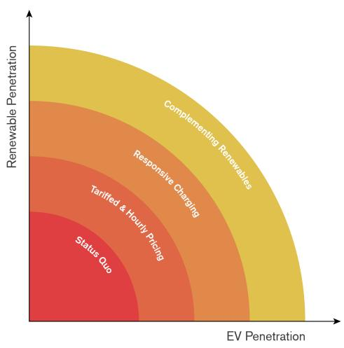
**Figure 9.4** Guideline for the evolution of schemes for controlling electric vehicle charging to become a participant in the energy system. With increasing penetrations of either EVs or renewables, more advance controls are required.
