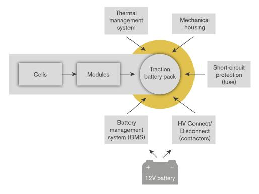
Figur 4.1 The traction battery system overview.
