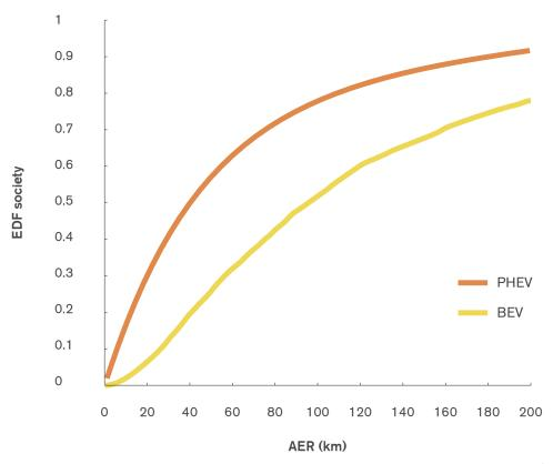
**Figure 10.4** The share of current private driving in Sweden possibly propelled by electricity (Electric Drive Fraction, *EDF*) as a function of battery range (AER) for PHEVs and BEVs, respectively. The charging is assumed to take place whenever a pause between trips is at least 10 hours (T = 10 h).
