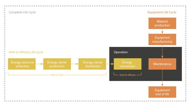
Figure 6.1 Simplified view of the well-to-wheels and equipment flows.
