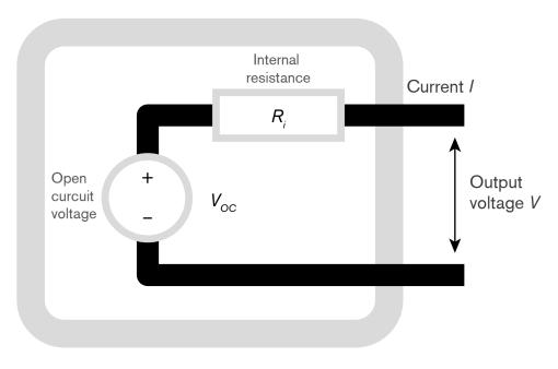
Output voltage  $V = V_{OC} - R_i I$ Power output  $P = V_{OC} I - R_i I^2$
