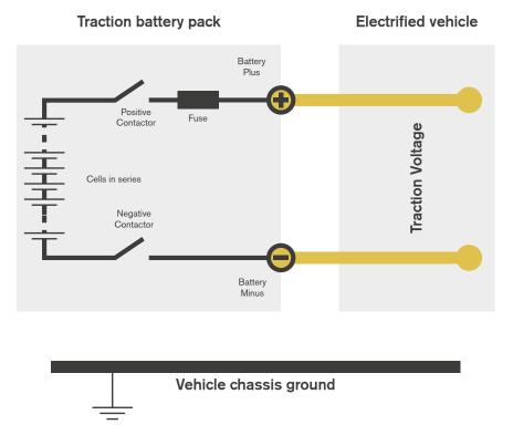
**Figur 4.4** Traction battery pack current path and the floating ground principle. If there are no insulation fault(s), there are no electrical connections between vehicle chassis ground and the battery poles.
