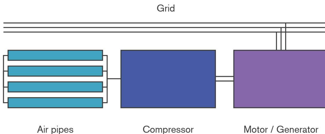
**Figure 5.5** Isothermal compressed air energy storage (above-ground)
