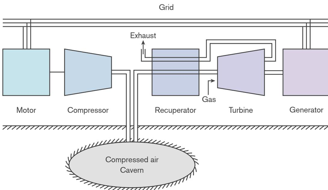
**Figure 5.4** Large-scale compressed air energy storage (underground)
