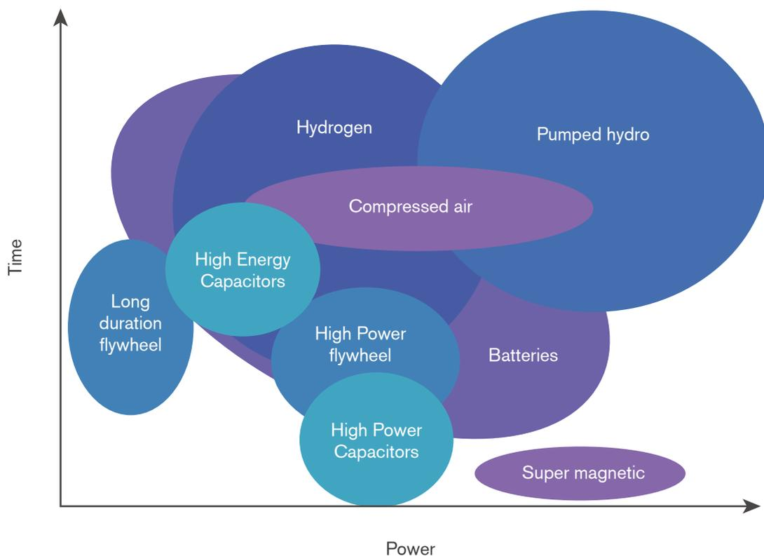
**Figure 5.1** Discharge time and different available capacity rates for storage technologies. The figure is only indicative. The time scale is logarithmic from seconds to months and the power scale is logarithmic from kW to GW.
