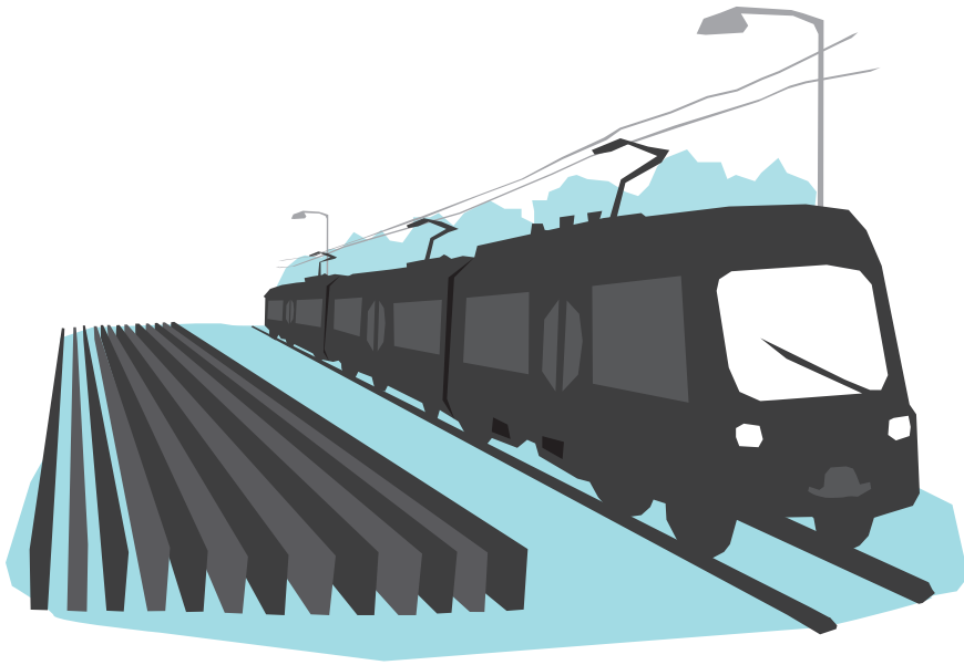
Roughness-based noise reduction using low parallel walls close to a tramway
