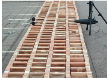
An array of nine parallel walls made from 1440 household bricks loosely stacked on edge (left). The same number of bricks made into a square-cell lattice (right).
