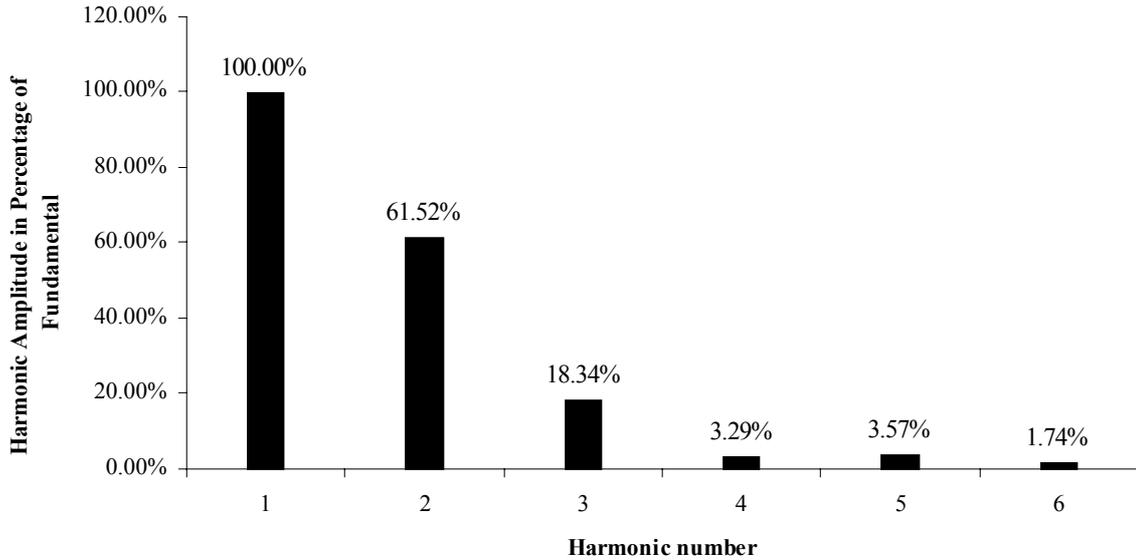
**Fig. 3.1d.** Odd line current harmonics normalized to the fundamental for the condition when the load is away from the distribution transformer resulting in lower harmonic currents due to higher input line impedance.
