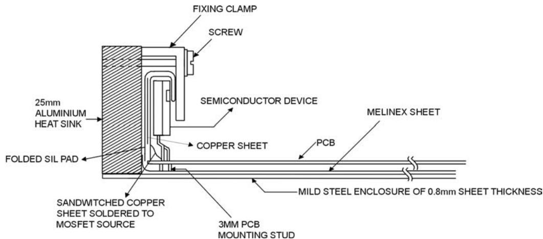
**Fig. 6.4a.** Mounting method of power semiconductor devices.
