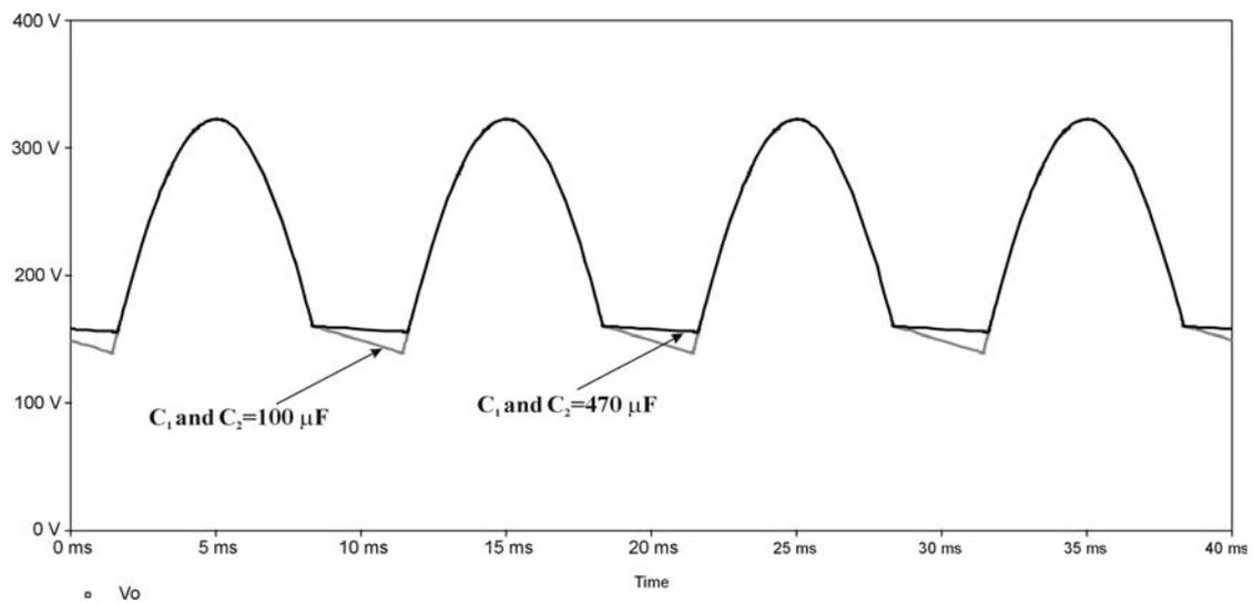
**Fig. 3.6c.** Simulated output voltage waveform with a 200 W constant power load for a valley fill rectifier based passive PFC circuit with capacitance values of 100  $\mu\text{F}$  and 470  $\mu\text{F}$ .
