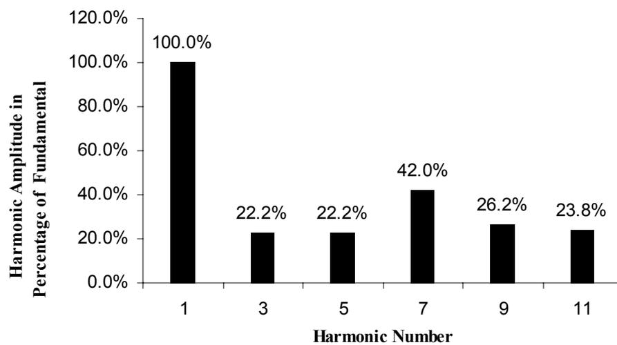
**Fig. 3.6d.** Odd line current harmonics normalized to the fundamental with a 200W constant power load for a valley fill rectifier based passive PFC circuit with capacitance value of 100  $\mu\text{F}$ .
