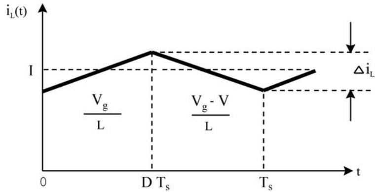
**Fig. 5.4** Inductor current wave form.
