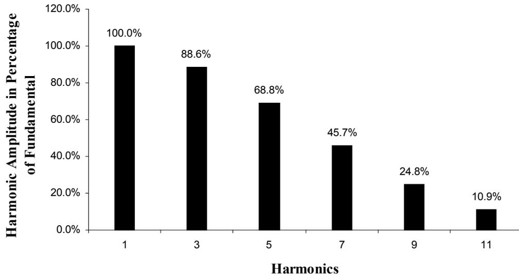
**Fig. 3.3c.** Odd line current harmonics normalized to the fundamental for a 200W constant power load with passive PFC circuit and 5 mH inductance.
