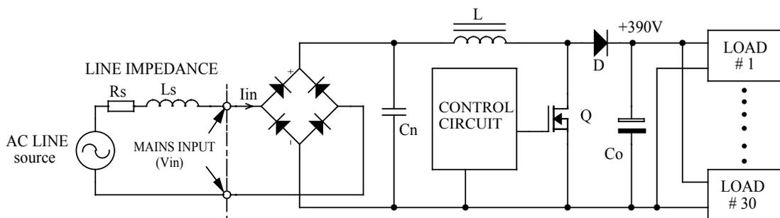
**Fig. 4.2.** The Common active PFC circuit scheme.
