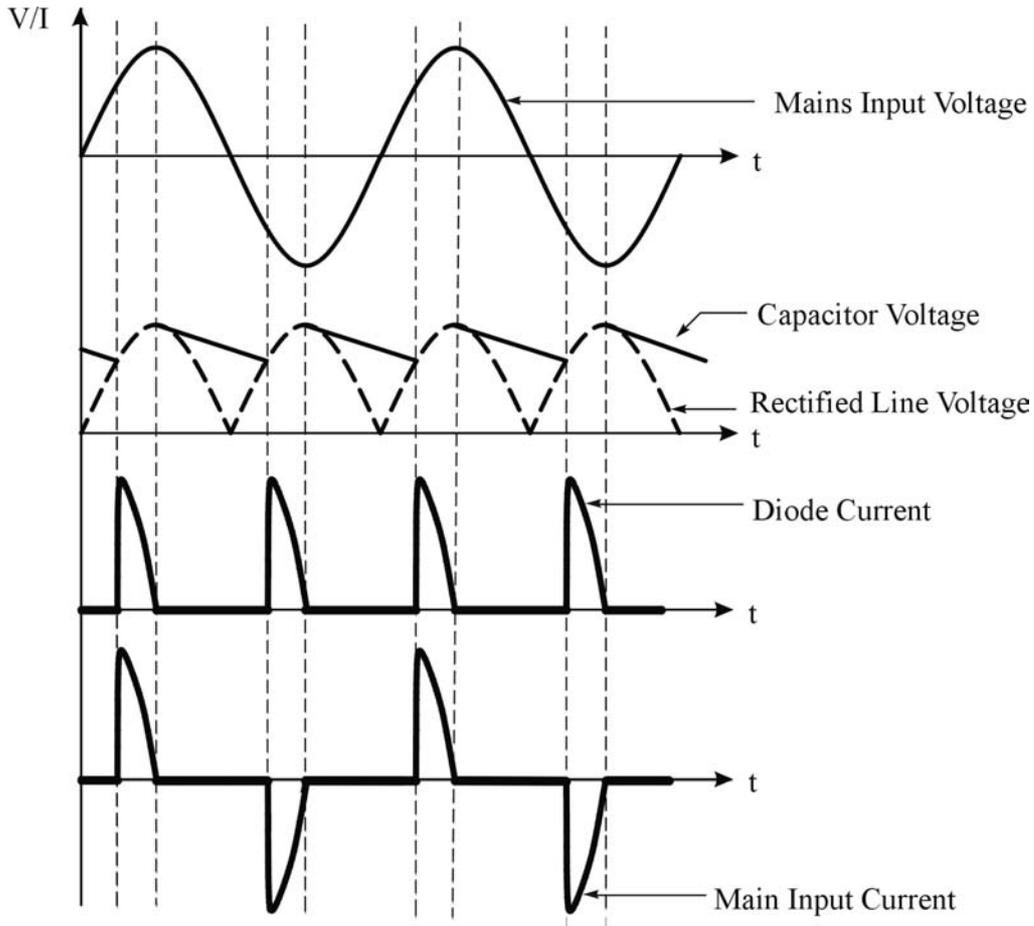
**Fig. 3.1b.** Typical line current and voltage waveforms.
