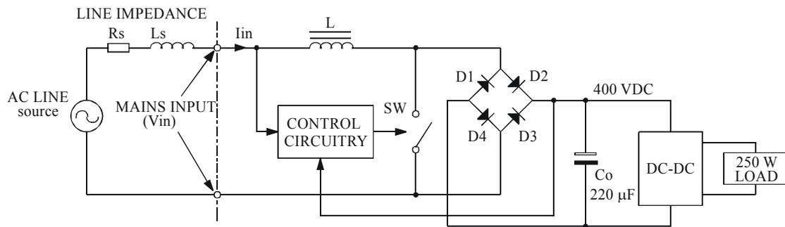
**Fig. 3.7a.** Typical schematic of a low frequency active PFC circuit.
