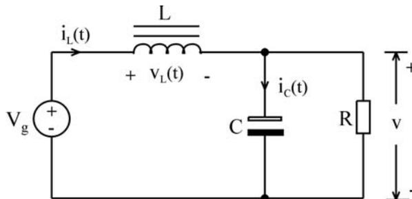
**Fig. 5.1c** Equivalent circuit of the CCM Boost converter when  $Q1$  turns OFF.
