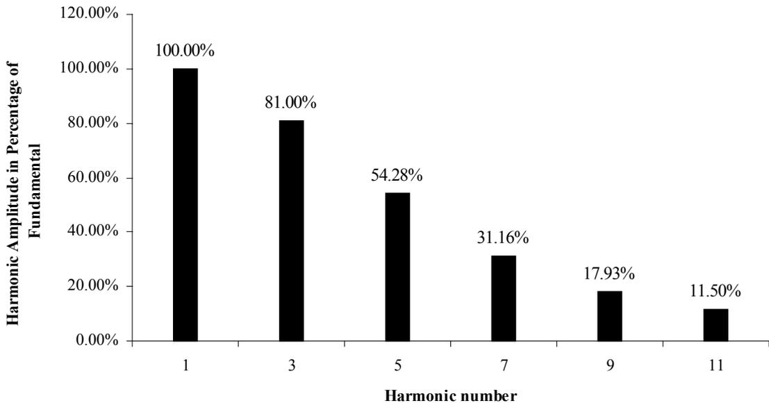
**Fig. 3.1c.** Odd line current harmonics normalized to the fundamental for the condition when the load is near the distribution transformer resulting in higher harmonic currents due to lower input line impedance.
