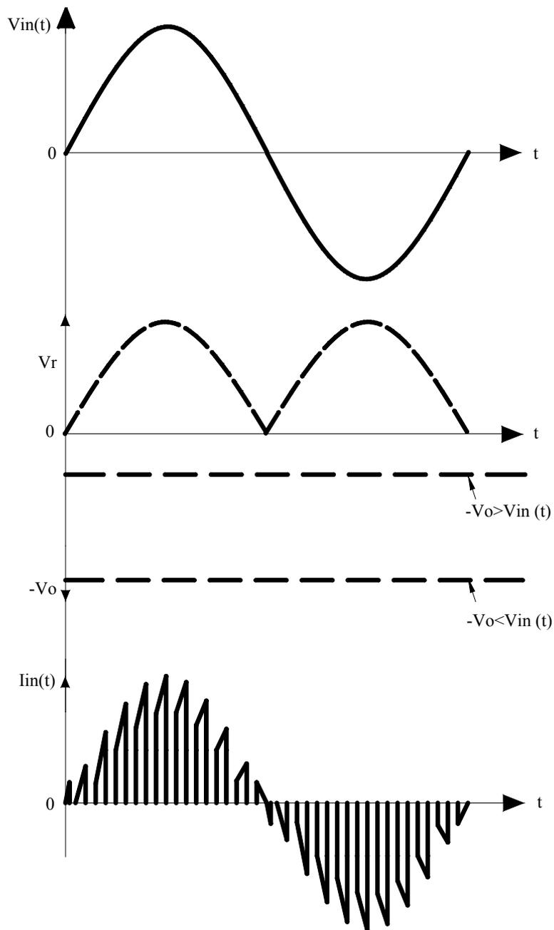
**Fig. 3.11b.** Current and voltage waveforms of buck-boost converter based PFC circuit.
