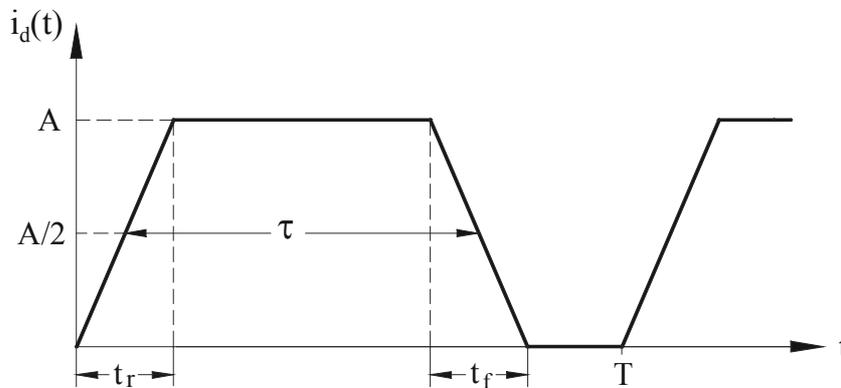
**Fig.5.10.** Periodic trapezoidal pulse train representing instantaneous drain current  $i_d$ .
