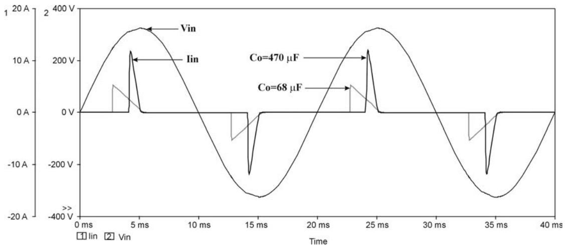
**Fig. 3.2b.** Simulated input voltage and current waveforms with filter capacitor  $C_o = 68 \mu\text{F}$  and  $C_o = 470 \mu\text{F}$ .
