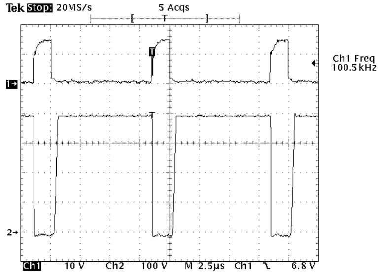
**Fig. 6.6.** MOSFET's gate and drain waveform for a smaller duty cycle.
