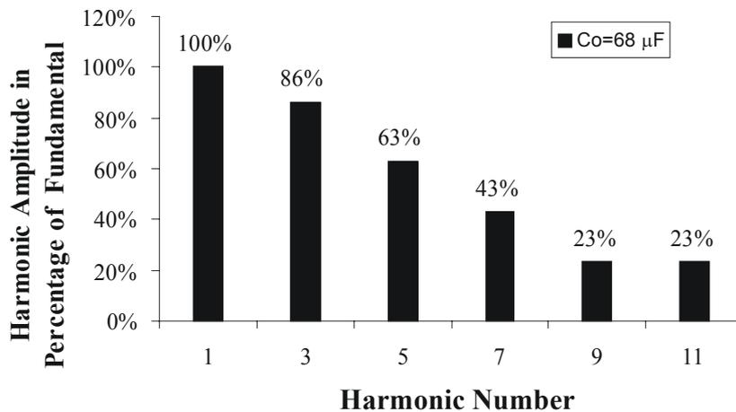
**Fig. 3.2d.** Odd line current harmonics normalized to the fundamental with filter capacitor  $C_o = 68 \mu\text{F}$ .
