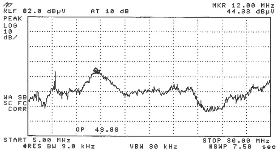
**Fig. 6.9 b.** Highest quasi-peak was recorded at 12.00 MHz and was of magnitude 43.88 dBµV.
