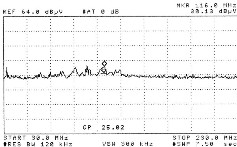
**Fig. 6.10** Highest quasi-peak was recorded at 116 MHz and was of magnitude 25.02 dBµV. This value excludes applicable antenna correction factor of about 10 and needs to be added to this result.
