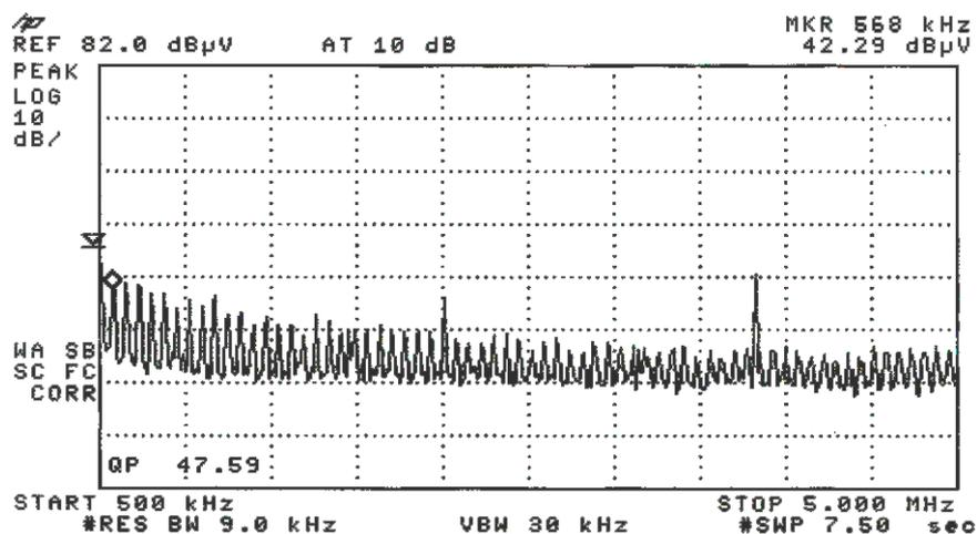
Fig. 6.9 b. Highest quasi-peak was recorded at 568 KHz and was of magnitude 47.59 dB $\mu$ V.
