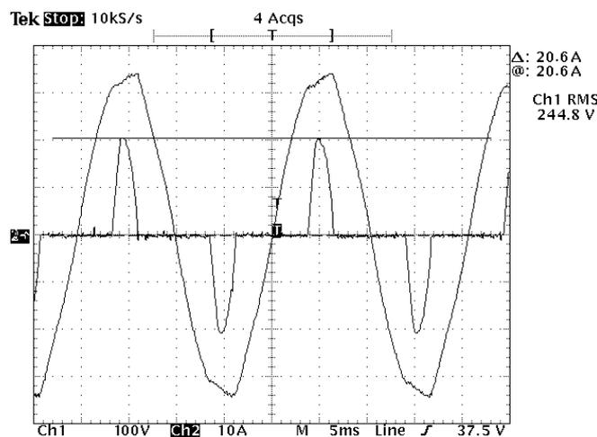
**Fig. 3.1e.** Voltage and current waveforms for a 1 kW constant power load for the condition when the load is near the distribution transformer resulting in higher input peak currents due to lower input line impedance.
