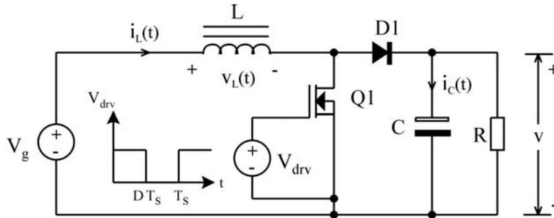
**Fig. 5.1a** Schematic of a CCM boost converter.
