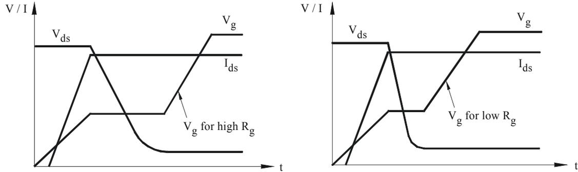
**Fig. 5.9.** Turn-on behavior for different gate resistance values.
