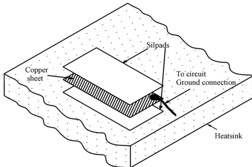
**Fig. 6.4b.** Representative diagram of a Faraday-shield insulator.
