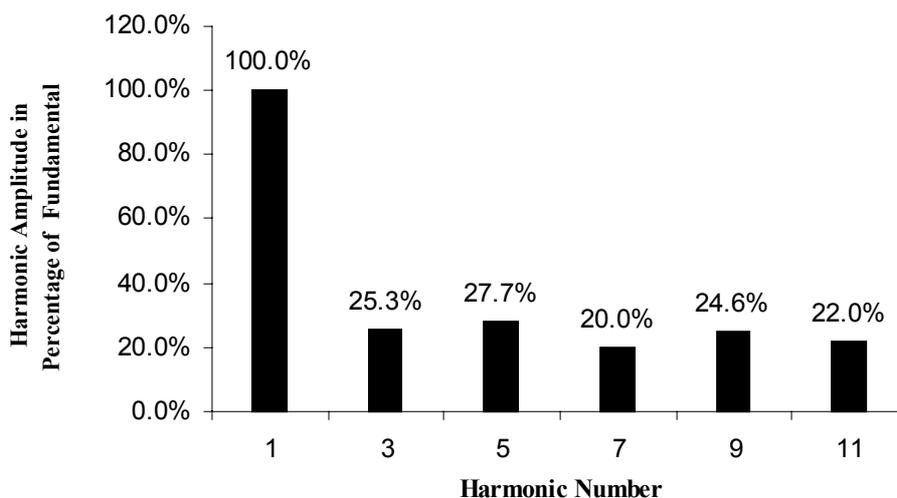
**Fig. 3.6e.** Odd line current harmonics normalized to the fundamental with a 200W constant power load for a valley fill rectifier based passive PFC circuit with a capacitance value of 470  $\mu$ F.
