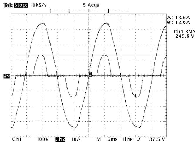
**Fig. 3.1f.** Voltage and current waveforms for a 1 kW constant power load for the condition when the load is away from the distribution transformer resulting in lower input peak currents due to higher input line impedance.
