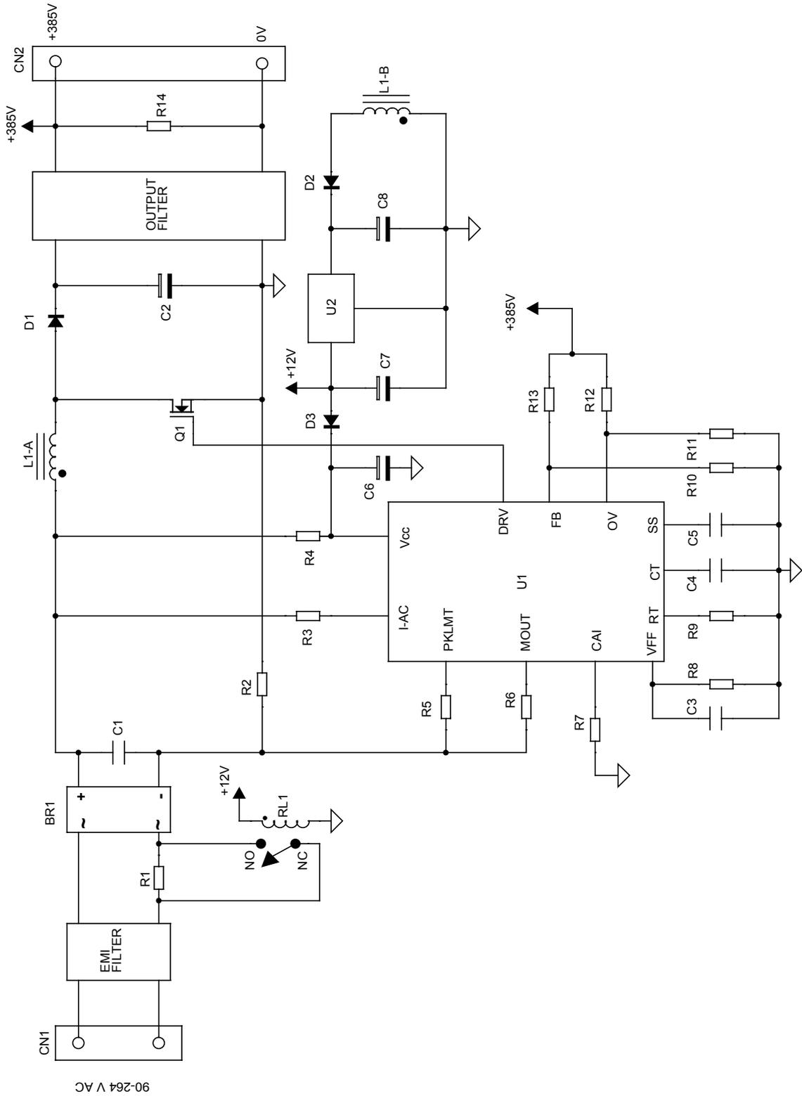
Fig 6.1. Block schematic of the 1200 W PFC circuit.
