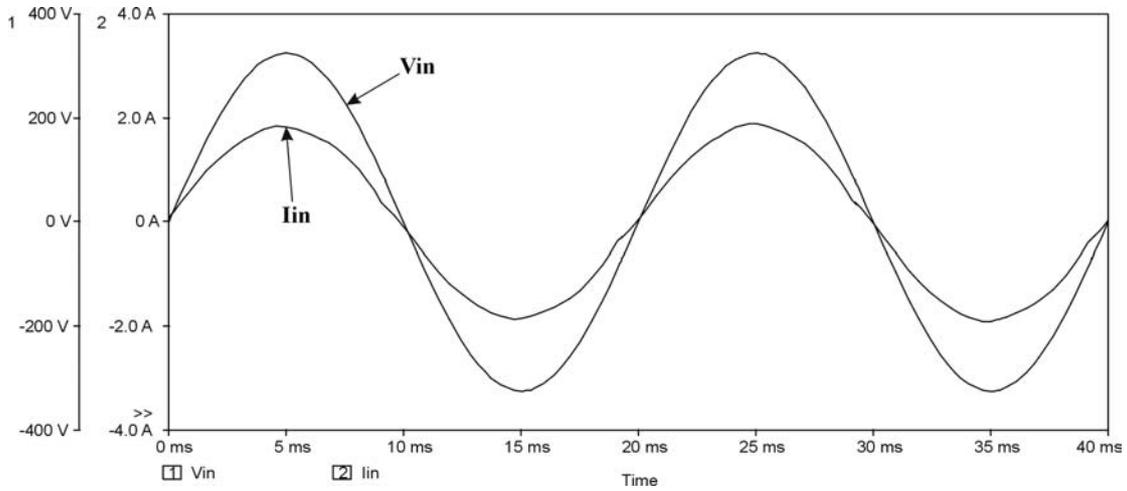
**Fig. 3.5b.** Simulated input current and voltage waveforms for a 300 W constant power load with harmonic trap filter for passive PFC circuit.
