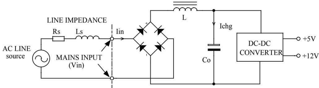
**Fig. 4.1** Simplified block diagram of the input circuit of most small electronic equipment.
