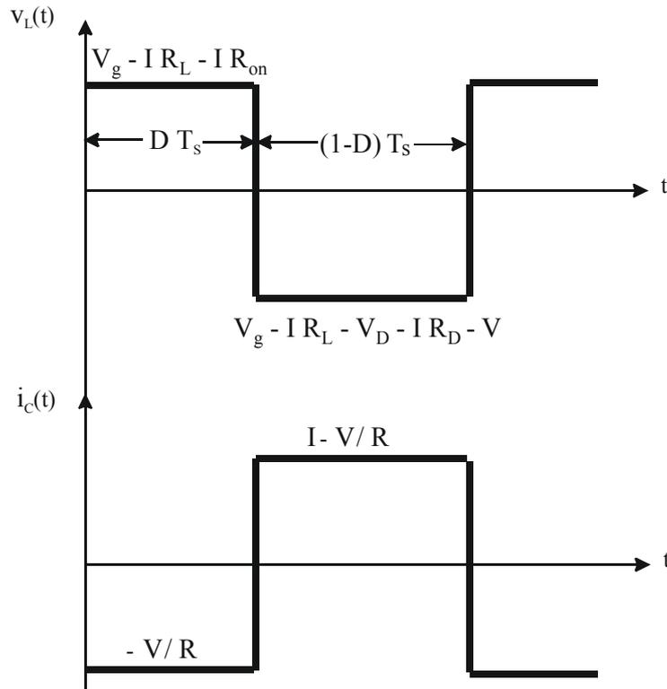
**Fig. 5.6** Inductor voltage and capacitor current wave forms.
