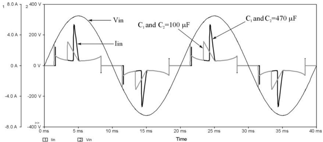
**Fig. 3.6b.** Simulated input current and voltage waveforms with a 200 W constant power load for a valley fill rectifier based passive PFC circuit with capacitance values of 100  $\mu\text{F}$  and 470  $\mu\text{F}$ .
