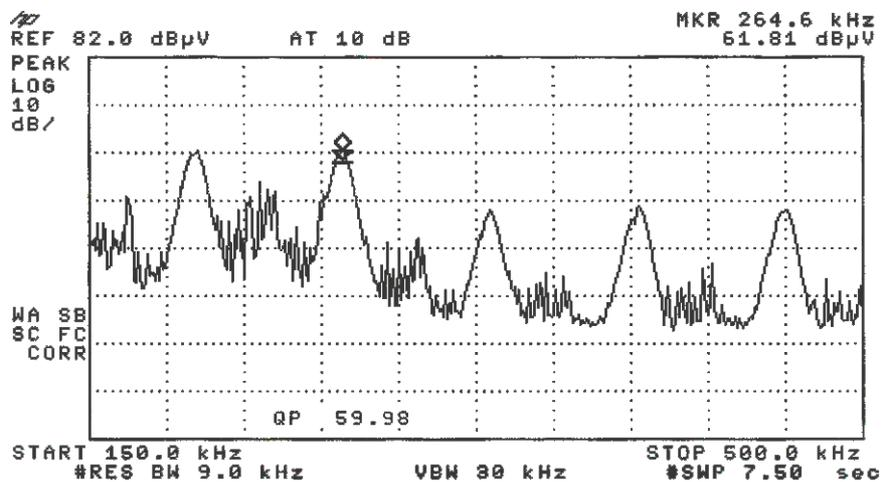
Fig 6.9 a. Highest quasi-peak was recorded at 264.6 kHz and was of magnitude 59.98 dB $\mu$ V.
