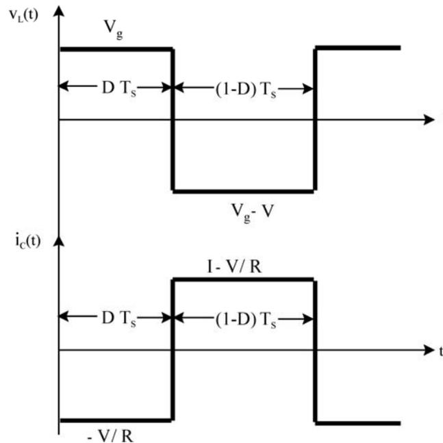
**Fig. 5.2** Inductor voltage and capacitor current wave forms.
