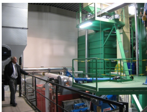
Figure 1. The BIOAGRO production facility from the inside. Pellet production to the right, and the BIOAGRO 1250kW BIOAGROFIRE pellet furnace to the right.
