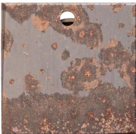
Figure 8.29 Optical image of the pre-oxidized alloy APMT (1 hour, 1100 °C) exposed for 1 corrosion exposure (O<sub>2</sub> + H<sub>2</sub>O + KCl at 600 °C for 24 hours).
