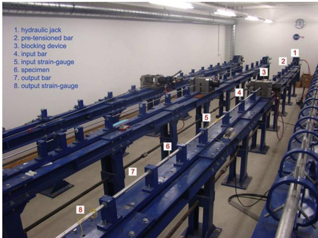
Figure 5: (Caverzan et al. 2012) used a Modified Hopkinson bar in order to investigate the material response at high strain rates.
