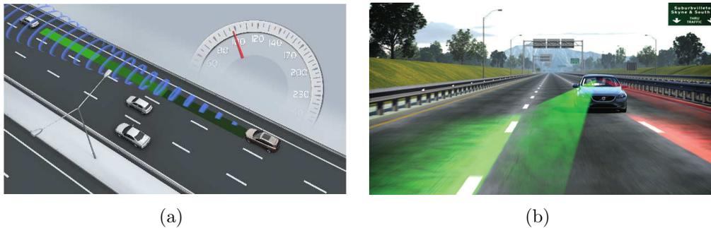
Figure 2.3: (a) A radar based ACC system (b) Lane keeping system.
