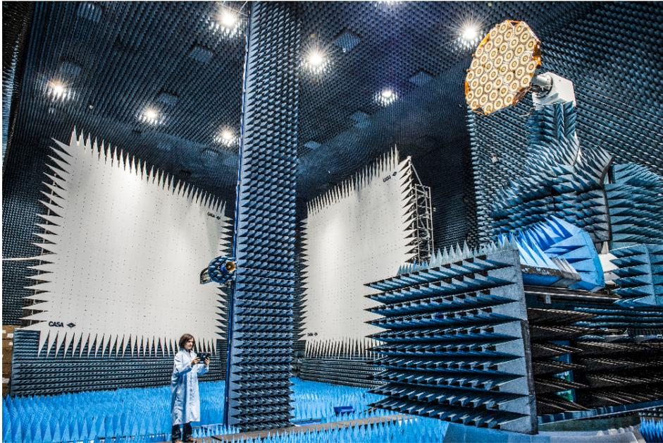
**Figure 2.19:** CATR setup located at ESTEC in Noordwijk, the Netherlands [69].
