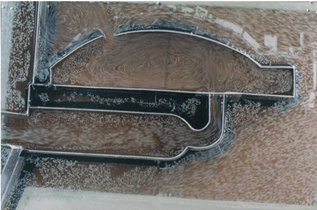
Figure 4: Flow pattern in a baking oven where the combustion chamber has a more rounded shape.
