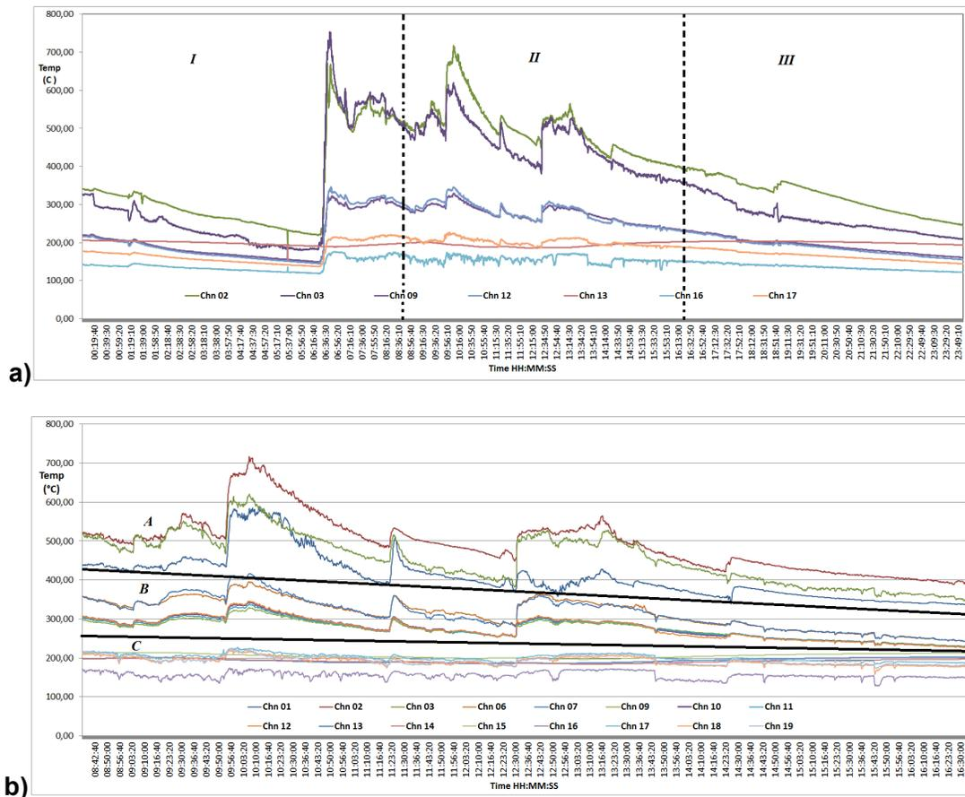
Figure 4.3.6: A typical temperature profile in a WFB, where a) is for the whole 24 hour period and b) is for the actual production period.
