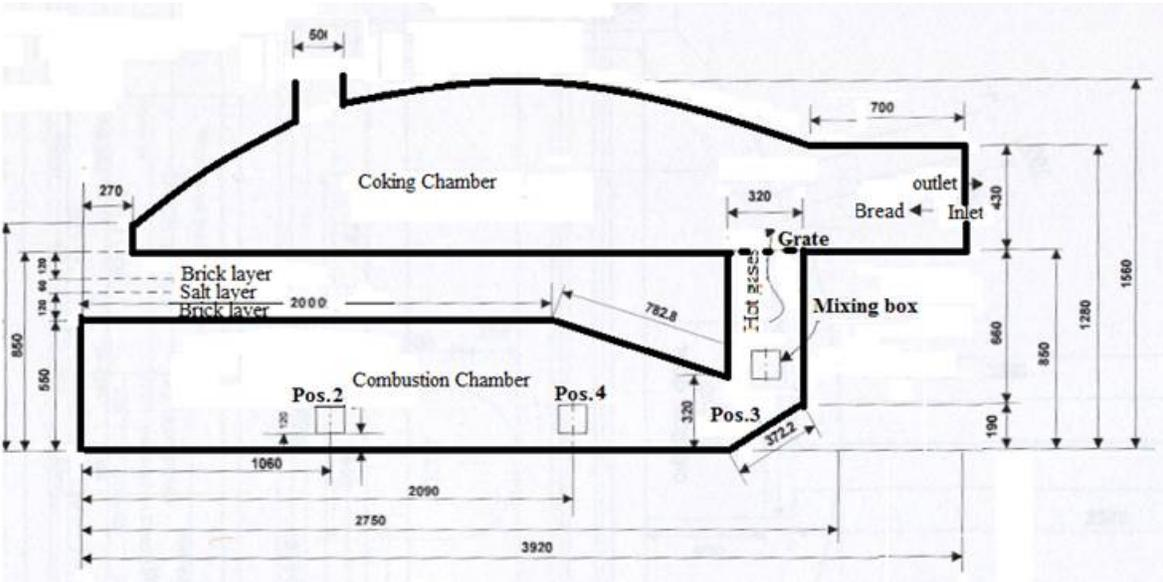
Figure 1: Technical design of the combustion chamber in a semi-direct wood-fired bakery oven, showing the positions at which the temperatures were measured.
