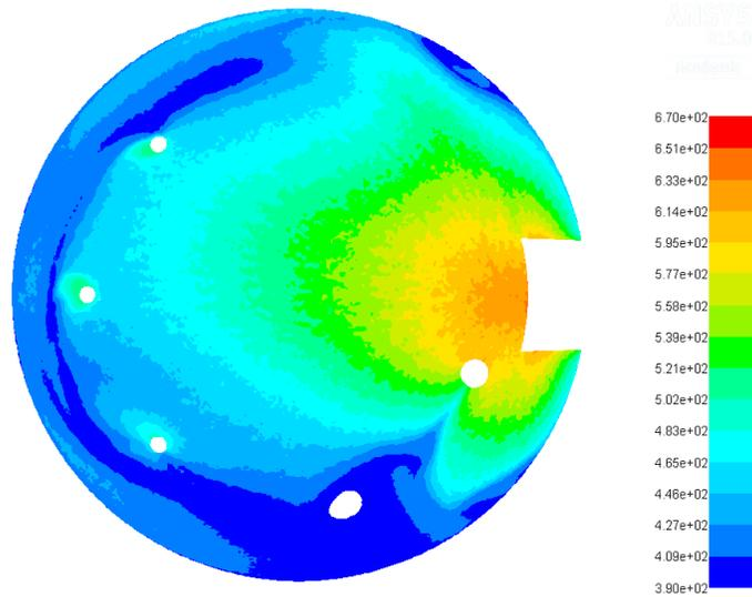
Figure 4.5.4: The temperature distribution along the oven ceiling
