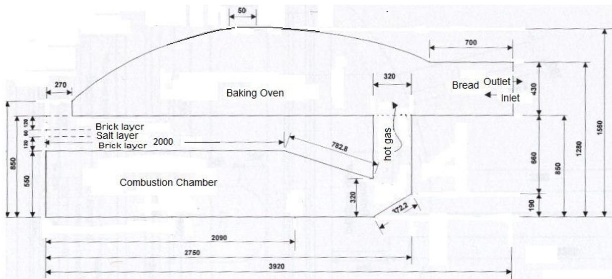
Figure 1.3.1: A longitudinal cross-section of a semi-direct bakery oven (a type of wood-fired bakery oven).
