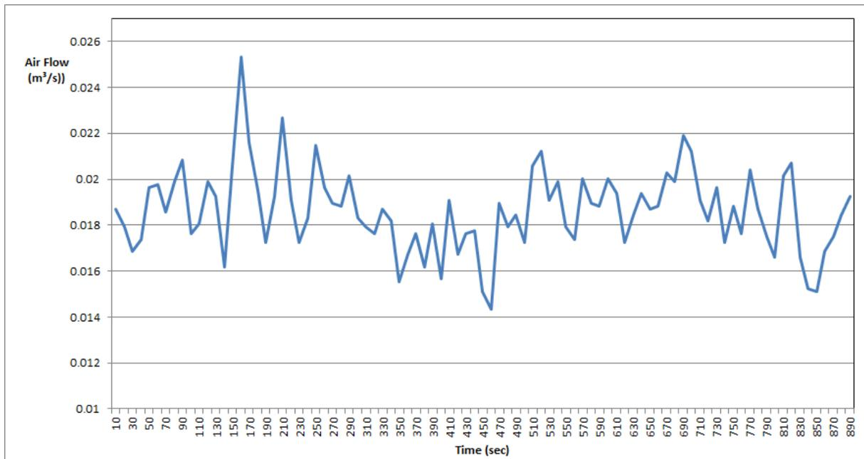
Figure 4.2.2. Variation of the rate of the air flow in the combustion chamber of a WFBO.
