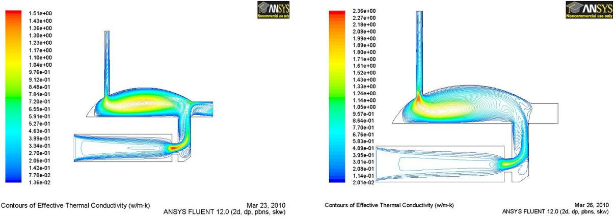
Figure 4.3.3: c) effective thermal conductivity, Flow patterns in a WFBO when the feeding door is opened (Left) and closed (right).
