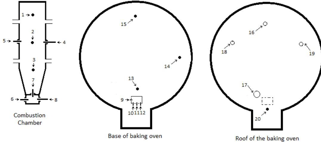
**Figure 3.4.2:** B. Location of the thermocouples in the WFBO.
