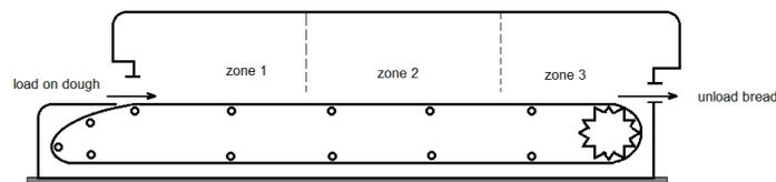
Figure 2.7.3: Schematic diagram of a tunnel-type (redrawn from Pyley 1973)
