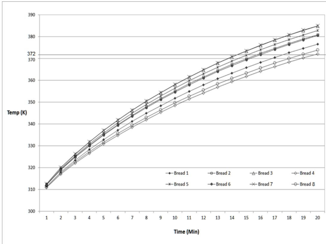
Figure 4.5.5: Average temperature profiles of the bread samples during the baking process. The line at 372 K corresponds to the required final bread temperature.
