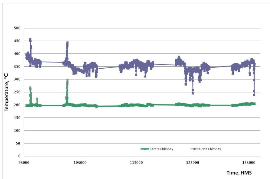
Figure 4.3.2: Graph of the temperature profile in the chimneys.
