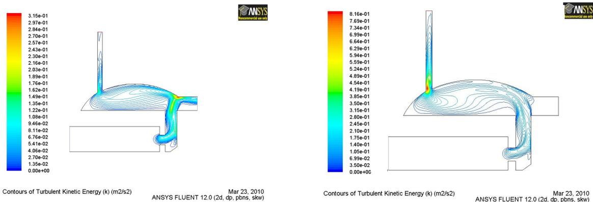
Figure 4.3.3: b) turbulent energy, Flow patterns in a WFBO when the feeding door is opened (left) and closed (right).
