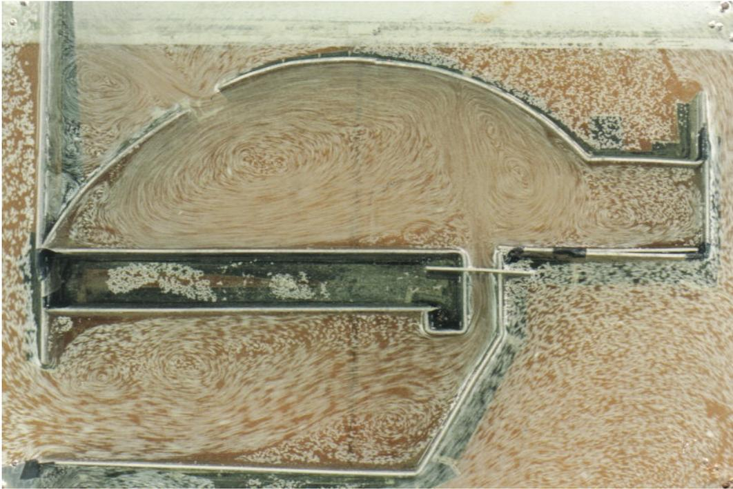
Figure 3: Flow pattern in a baking oven, where the combustion chamber is rectangular in shape
