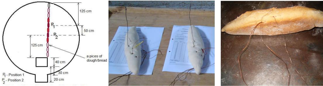
*Figure 3.1.1.B:* Schematic representation of the positions of the loaves in the baking chamber and the techniques used to study the temperature profile in the bread baking process (dough and bread, respectively)
