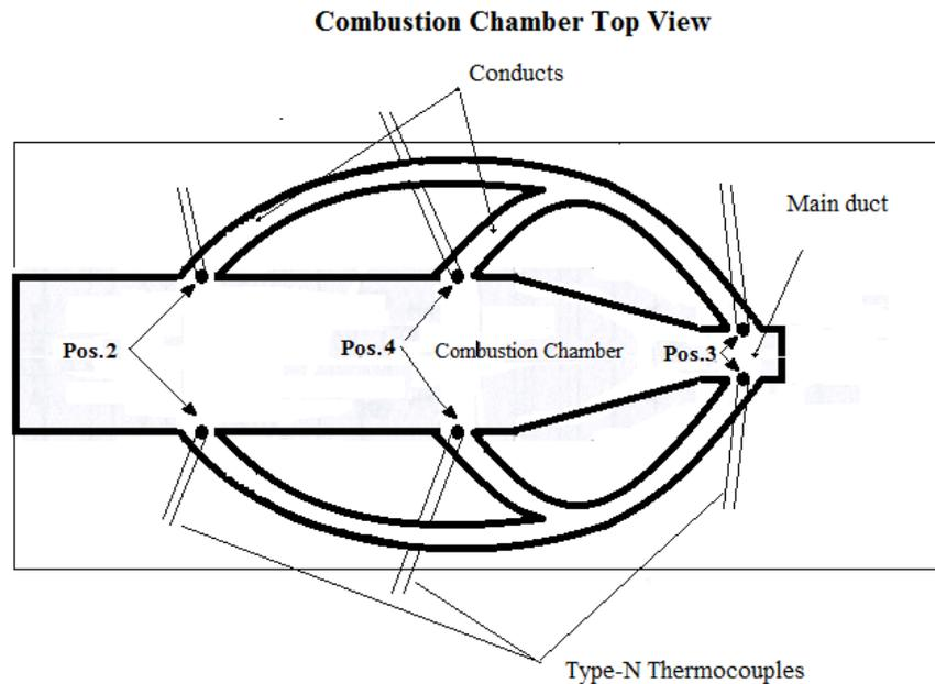
Figure 3.1.1.A: Schematic representation of the position in which the combustion temperatures were measured.
