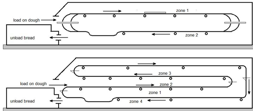
Figure 2.7.2: Schematic diagram of a single lap and a double lap oven (redrawn from Pyley 1973)
