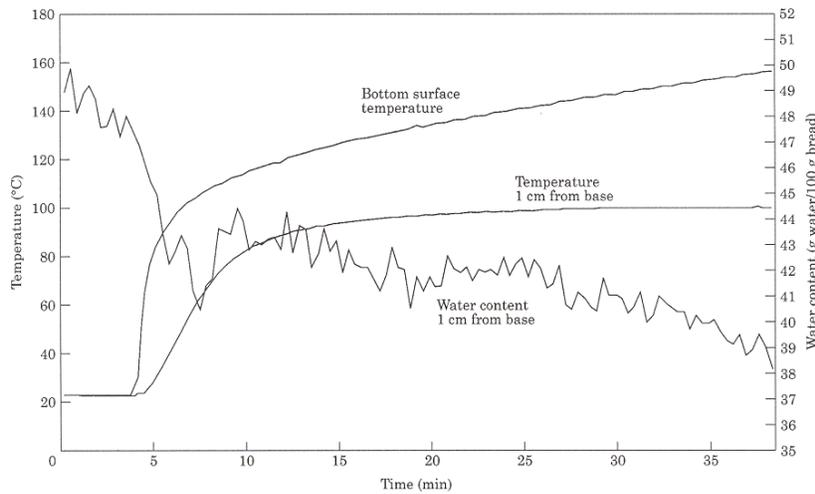
Figure 2.5.1: c) Water content and temperature profile in the bottom surface (from Thorvaldsson and Skjoldebrand 1998).
