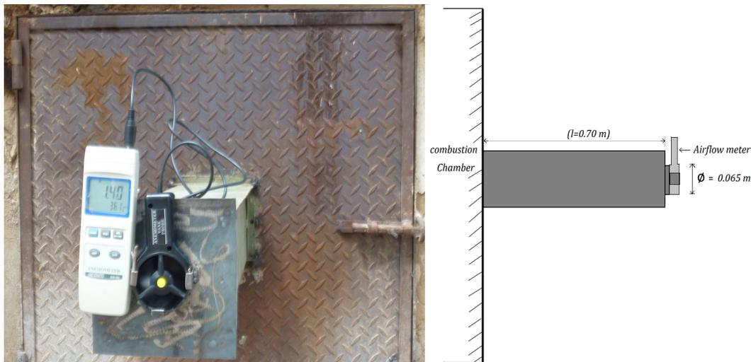
Figure 3.4.3: Measurement of the airflow entering the combustion chamber. Left: a photograph. Right: the arrangement.
