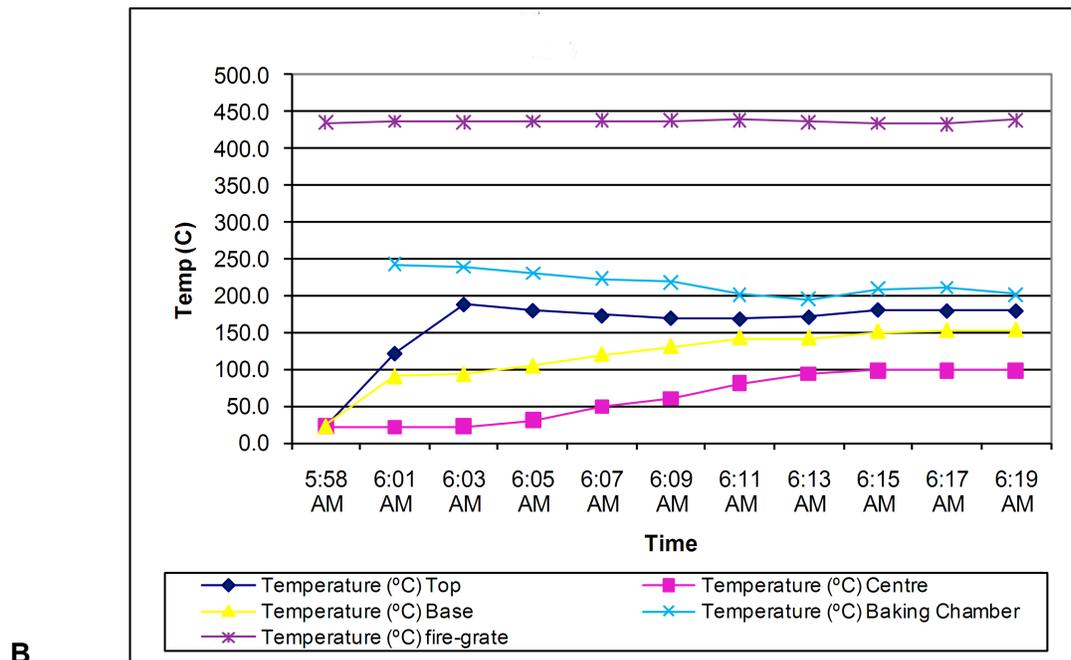
Figure 4.4.3. A. Temperature profile measured at position P2 in a semi-direct WFBO when the bread is baked at the fire-grate temperature 450°C. B. Temperature profile measured at position P1 in a semi-direct WFBO when the bread is baked at the fire-grate temperature 350°C.
