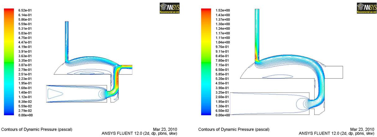
Figure 4.3.3: d) dynamic pressure, Flow patterns in a WFBO when the feeding door is opened (left) and closed (right)
