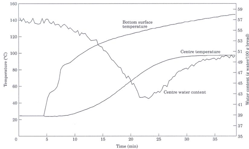
Figure 2.5.1: b) Water content and temperature profile in the centre (from Thorvaldsson and Skjoldebrand 1998)
