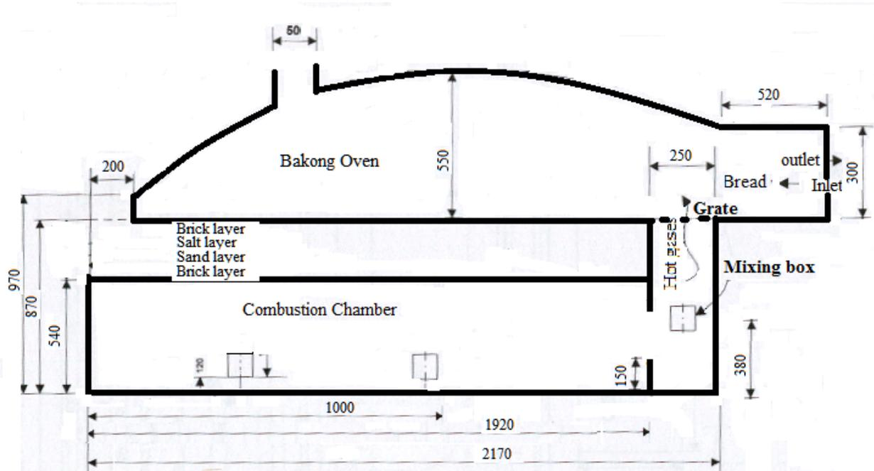
**Figure 3.4.2:** A. The technical design of the wood-fired bakery oven by taking a longitudinal cut at the central section of the WFBO.
