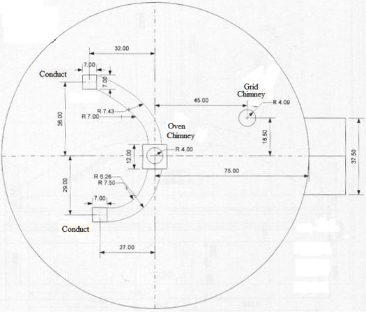
Figure 2: Arrangement of the chimneys above the baking oven in a the wood-fired bakery oven
