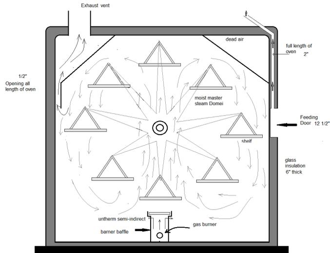
Figure 2.7.1: Cross-section of a reel oven (redrawn from Pyley 1973)
