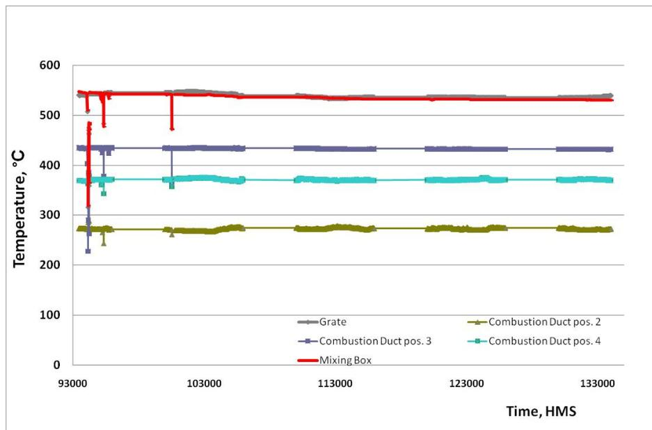
Figure 4.3.1: Graph of the temperature profile in the combustion chamber.
