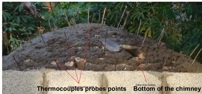
Figure: 3.4.1:b) The distribution of the probes along the baking chamber.
