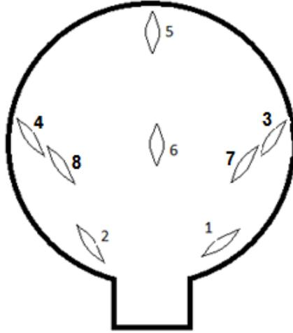
Figure 3.4.4: Location of the samples within the oven.
