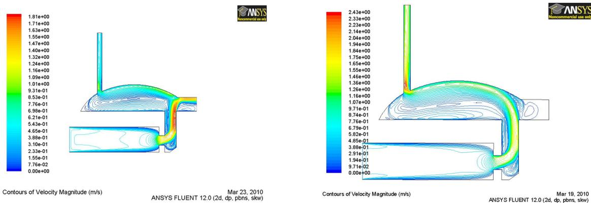
Figure 4.3.3: a) Velocity, flow patterns in a WFBO when the feeding door is opened (left) and closed (right).
