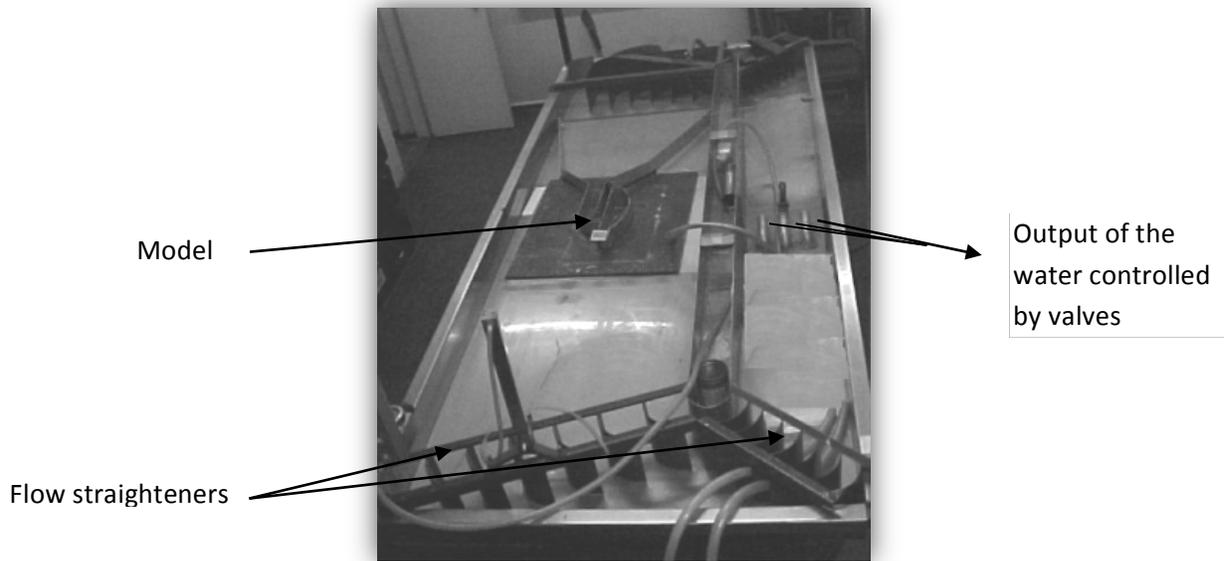
Figure 3.2.1: The bi-dimensional water table used in the physical simulation studies.
