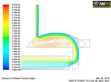
Contours of Stream Function (kg/s) Mar 26, 2010 ANSYS FLUENT 12.0 (2d, sp, psm, ssw)
