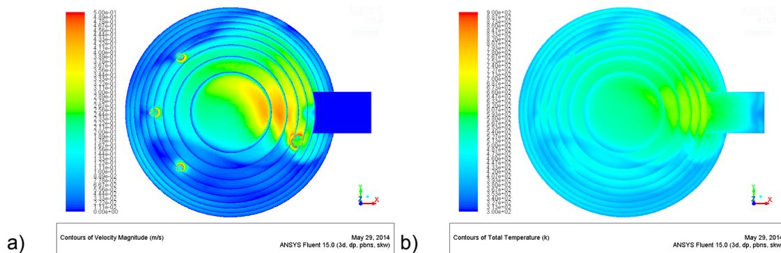
Figure 4.5.1: Velocity (a) and (b) temperature profiles in entire baking oven.
