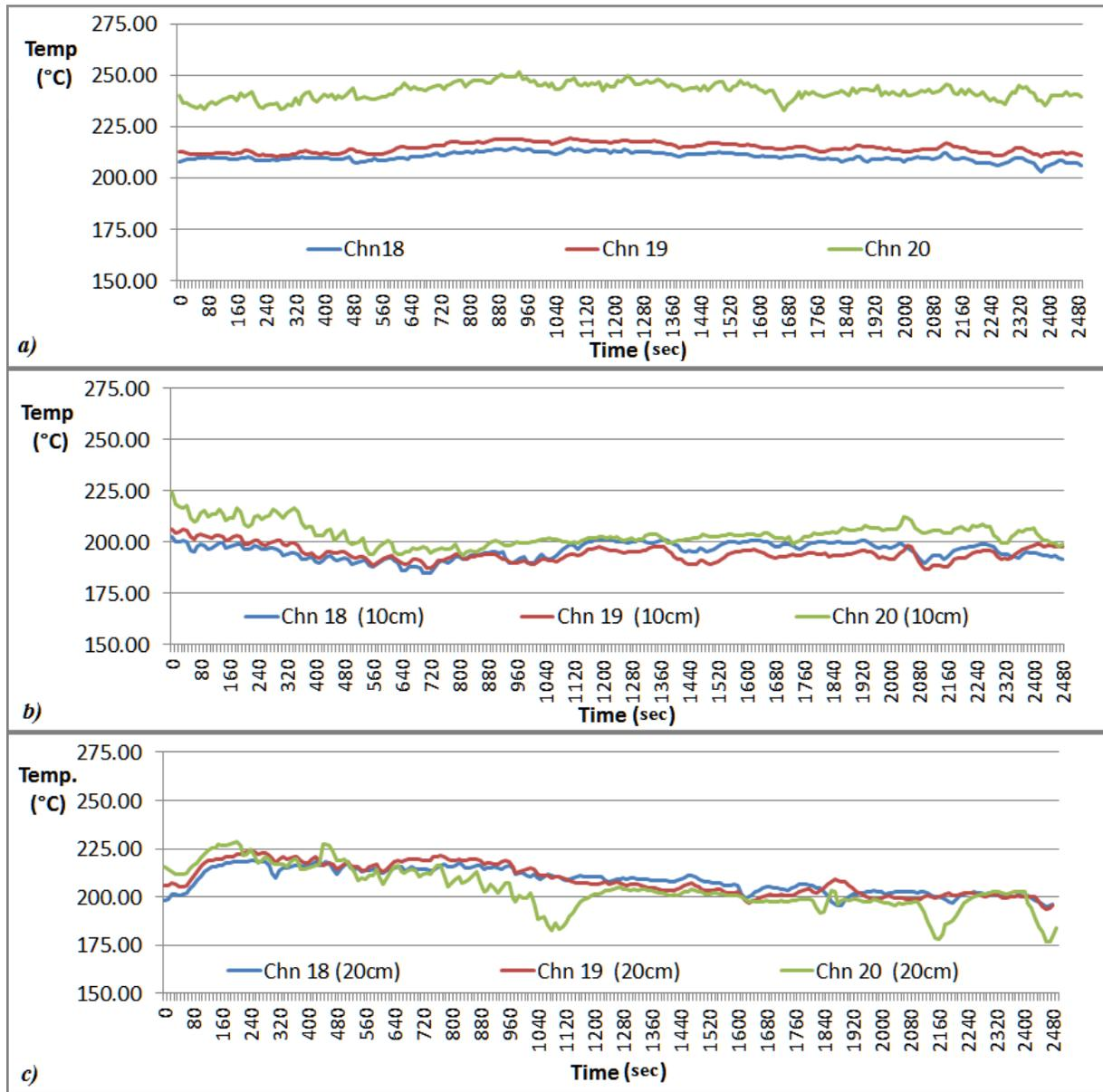
**Figure 4.3.7:** Temperature profiles at different distances from the ceiling of the baking oven during the baking process.
