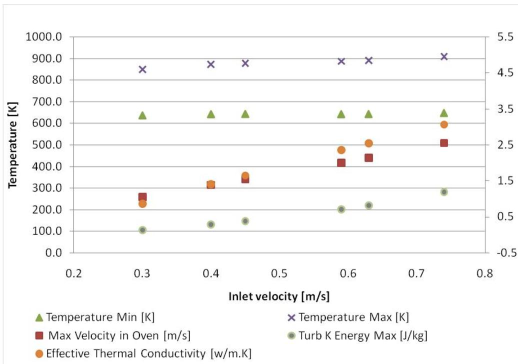
Figure 4.3.4: The impact of velocity on several parameters (Temperature at left Y Axis and other parameters at right Y Axis)
