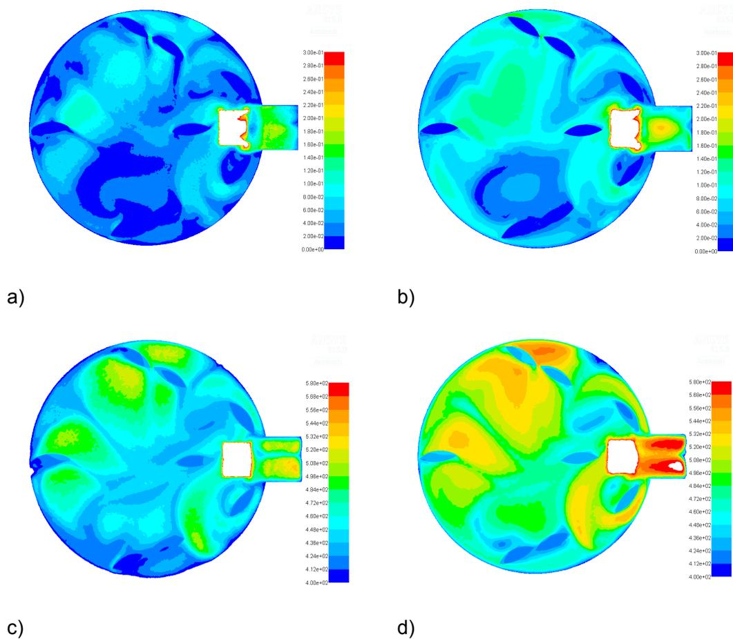
Figure 4.5.2: Velocity and temperature profiles in the baking oven containing bread. Velocity profile at a height above the oven base of a) 1 cm and b) 5 cm. Temperature profile at a height above the oven base of c) 1 cm and d) 5 cm.
