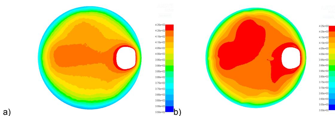
Figure 4.5.3: Temperature distribution in a WFBO a) in the salt layer and b) at the base of the oven.
