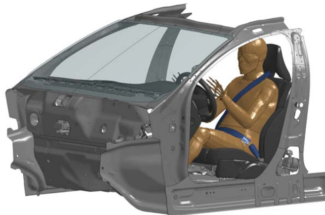
Fig. 4. Interior vehicle model with THUMS in the driver position
