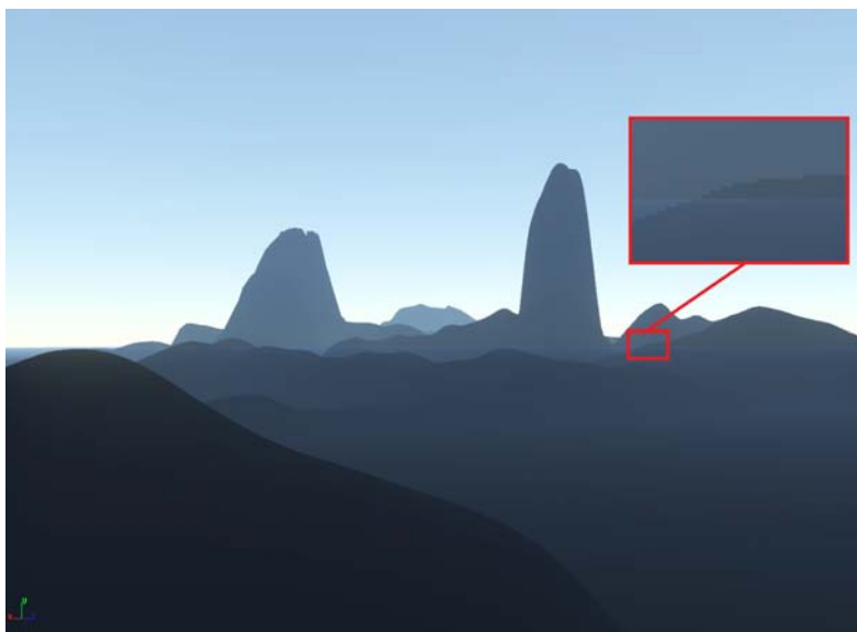
Figure 16: Aerial Perspective inscattering, with artifacts due to the discontinuity at the horizon.
