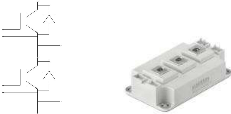
Fig. 3.2: The symbols and picture of the IGBT modules of the DAB converter
