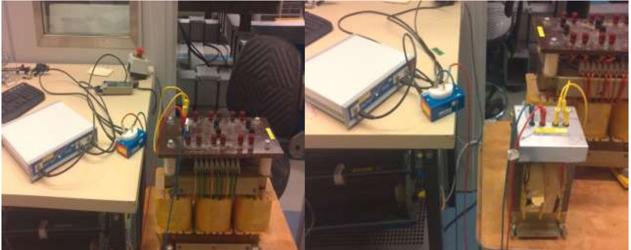
Fig. 3.6: leakage inductance measurement of the single and three phase transformers by using Bode 100
