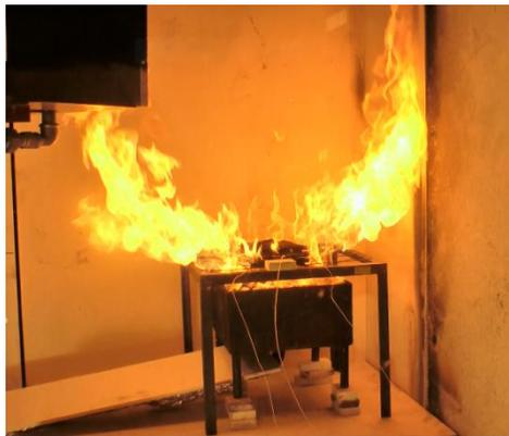
Fig. 6. Outbursts from EiG 100% SOC (test 1).
