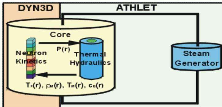
In the second type of coupling the whole core is cut out of the ATHLET plant solution and is completely modeled by DYN3D (external coupling), making use of its TH (FLOCAL) module.
