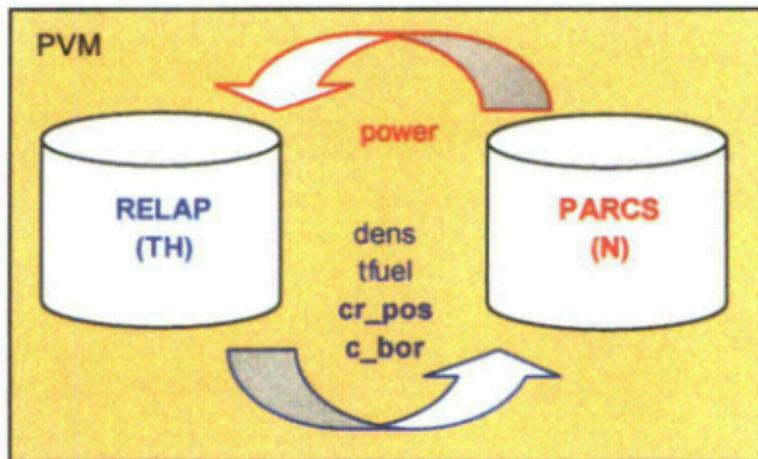
In RELAP5/KAPROS, the super-cell model from KAPROS is coupled with the TH system code RELAP5, being improved for High Performance Light Water Reactor (HPLWR) applications. The RELAP5 input model describes the whole reactor system, including a one-channel representation for the core. In this
