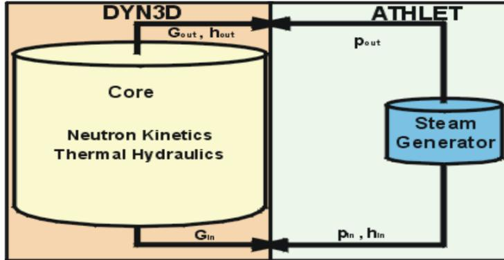
For the third type of coupling, the TH is split into two parts: the FLOCAL core model of DYN3D and the ATHLET model of the core and cooling system. Boundary conditions are provided to the DYN3D by the core TH solution of ATHLET.
