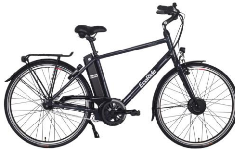
Figure 8. Example of typical commercial E-bike. The motor is in this case placed in the hub of the front wheel (rated at 250 W) and the battery and its electronics is enclosed in the black box right of the rear wheel. Typically, there is also a small control panel on the handles. Reproduced with permission of EcoRide (2014).
