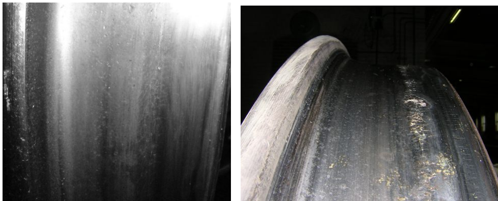
Figure 3. Examples of low (left) and high (right) severity of surface initiated rolling contact fatigue in zone 1.
