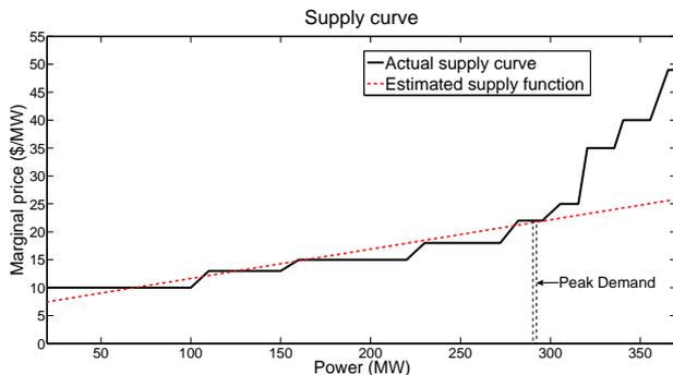
Figure 3.5: Supply curve for modified IEEE 30-bus system
