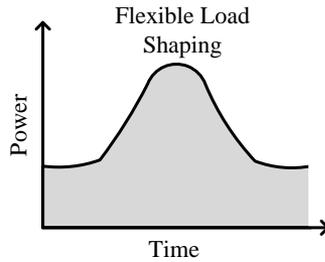
Figure 2.7: Change in load profile due to load shaping
