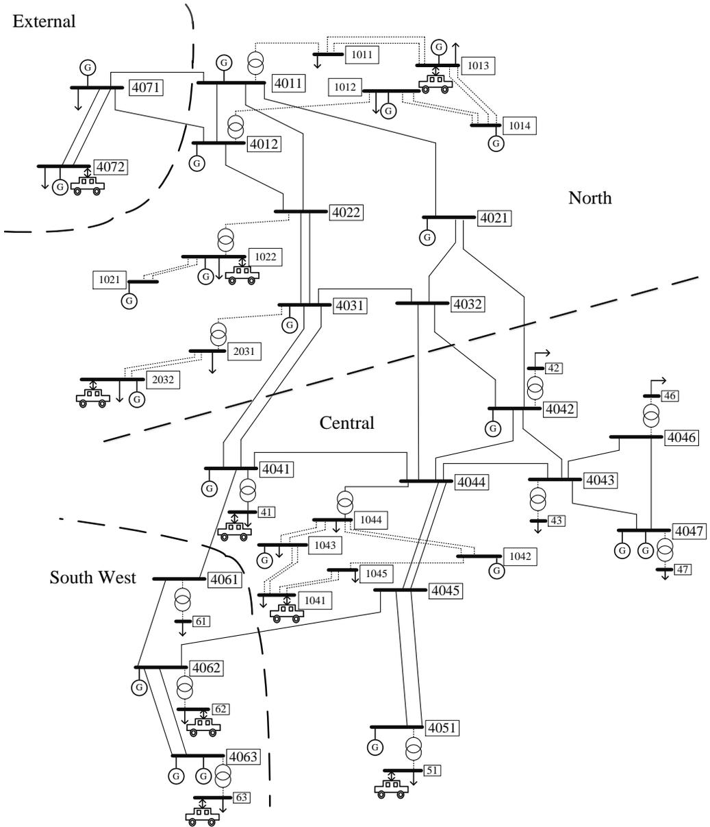
Figure 4.2: Nordic 32-bus Test System [69]
