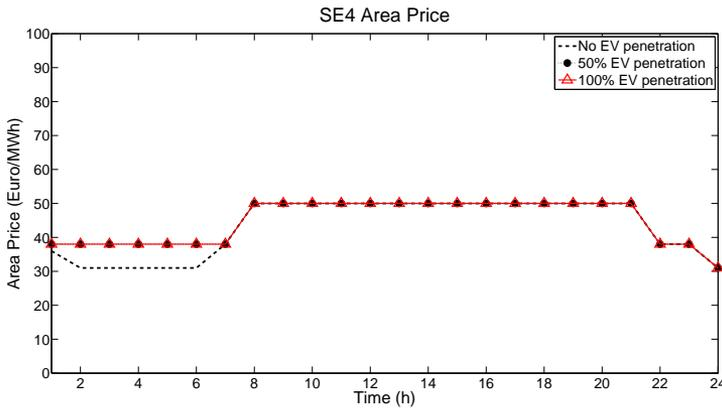
Figure 3.21: Constrained case result- SE4 area price at different EV penetration levels
