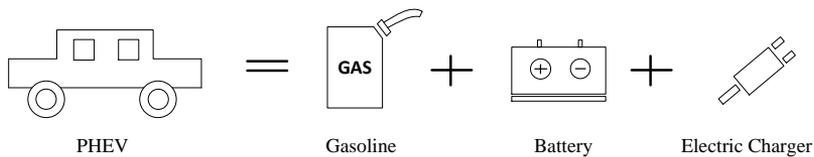
Figure 2.13: Plug-in hybrid electric vehicle
