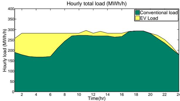
Figure 3.9: JSM result- system demand at zero and 100% EV penetration
