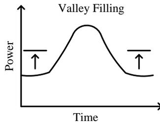
Figure 2.5: Change in load profile due to valley filling
