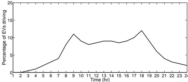
Figure 5.5: Driving pattern of EVs based on conventional vehicle data [48], [72]
