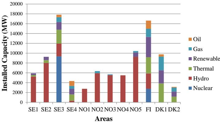
Figure 3.13: Generating capacity distribution by bidding area in the Nordic region
