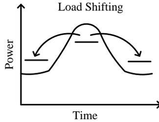
Figure 2.6: Change in load profile due to load shifting
