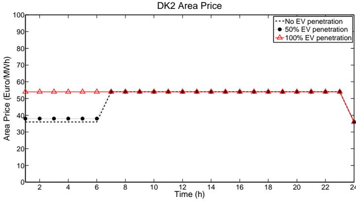
Figure 3.22: Constrained case result- DK2 area price at different EV penetration levels
