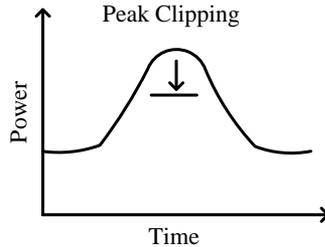
Figure 2.4: Change in load profile due to peak clipping
