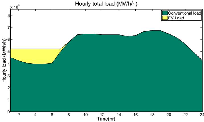
Figure 3.17: Unconstrained case result- total load at 100 % EV penetration
