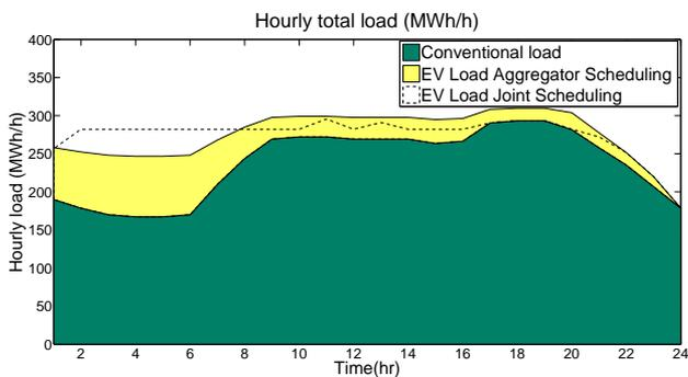
Figure 3.11: ASM and JSM comparison result- system demand at zero and 100 % EV penetration
