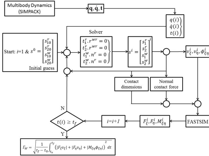
**Fig. 6:** Wear post-processor algorithm.
