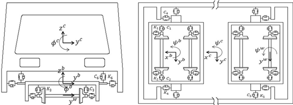
**Fig. 1:** One car vehicle model A.
