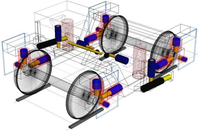
**Fig. 2:** Bogie corresponding to the vehicle model C developed in SIMPACK.
