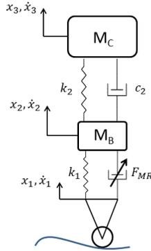
**Fig. 7:** Application of MR dampers in bogie primary suspension.
