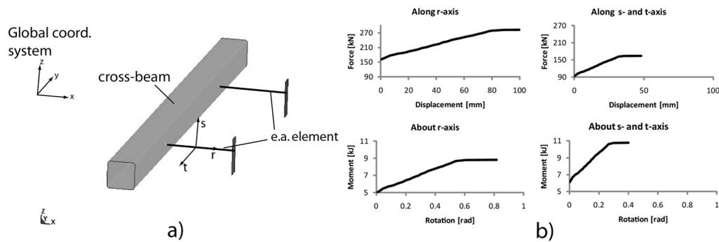
Figure 7: Model of simplified e.a. FUPD: (a) e.a. FUPD consisting of FUPD cross-beam and FUPD e.a. elements (modelled as springs) and (b) force/moment versus displacement/rotation characteristics of the e.a. elements (springs)
