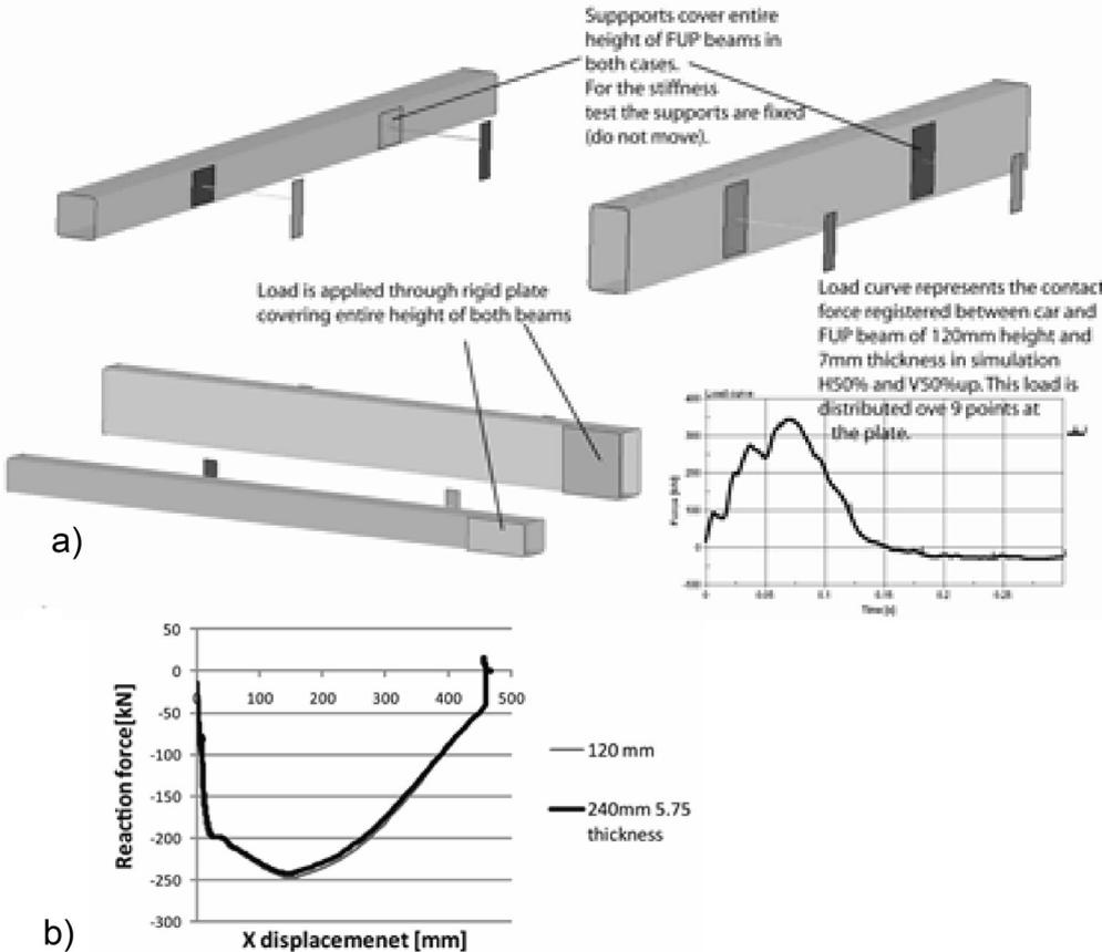
Figure 9: a) Set-up of the bending test simulation with a loading curve; b) Displacement of the FUPD cross-beam end for the different cross-beam heights under bending test
