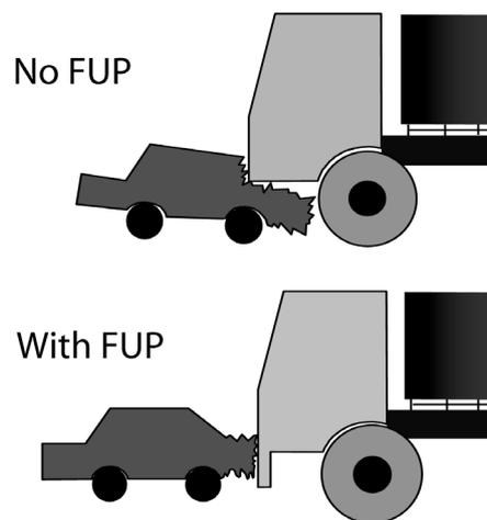
Figure 2: *Motivation for Front Underrun Protection (Wrige, 2003)*
