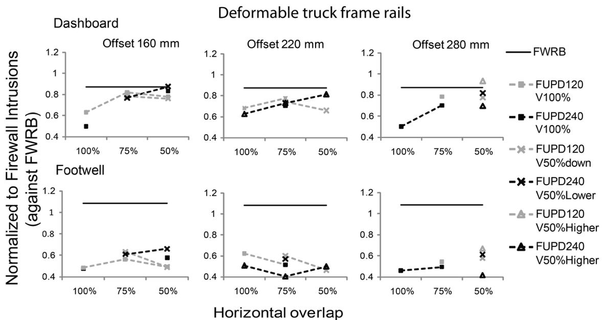
Figure 12: Calculated intrusions of the dashboard and footwell of the car impacting the truck with deformable frame rails
