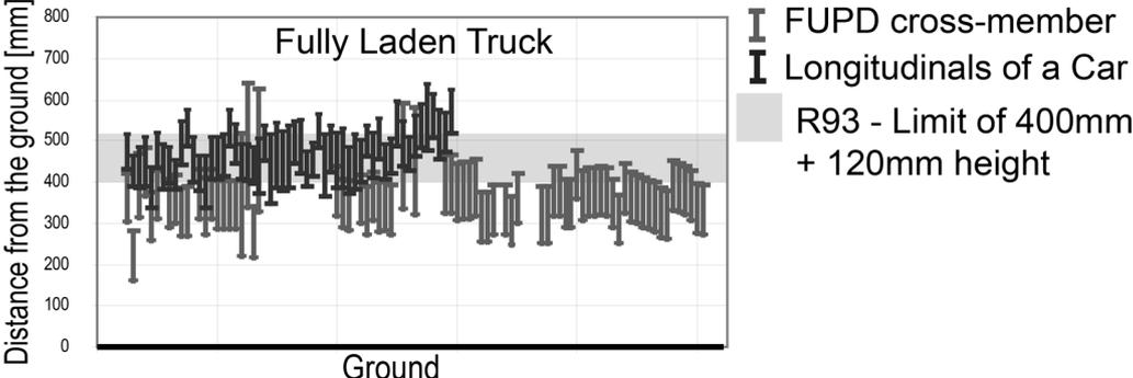
Figure 5: A graphical presentation of relative position between car longitudinals and FUPD cross-beam for fully laden trucks based on the geometrical database
