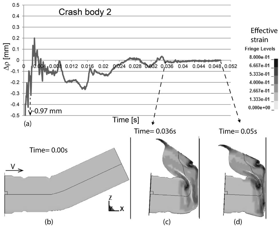
Figure 14: *Crash Body 2. (a) RED curve, (b) initial state just before impact, and states at approximate time points when (c) the buckling stops and (d) displacement reaches its maximum value, respectively at lower row with effective strain fringe pattern*
