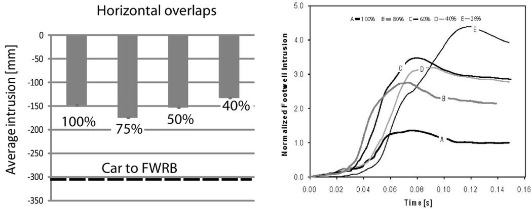
Figure 8: a) Average intrusions from car to e.a. FUPD for different horizontal overlaps in comparison to intrusions caused by impact into FWRB b) Normalized (to intrusions for full overlap) footwell intrusions from car-to-car simulations for different horizontal overlaps (complementary Paper 1)
