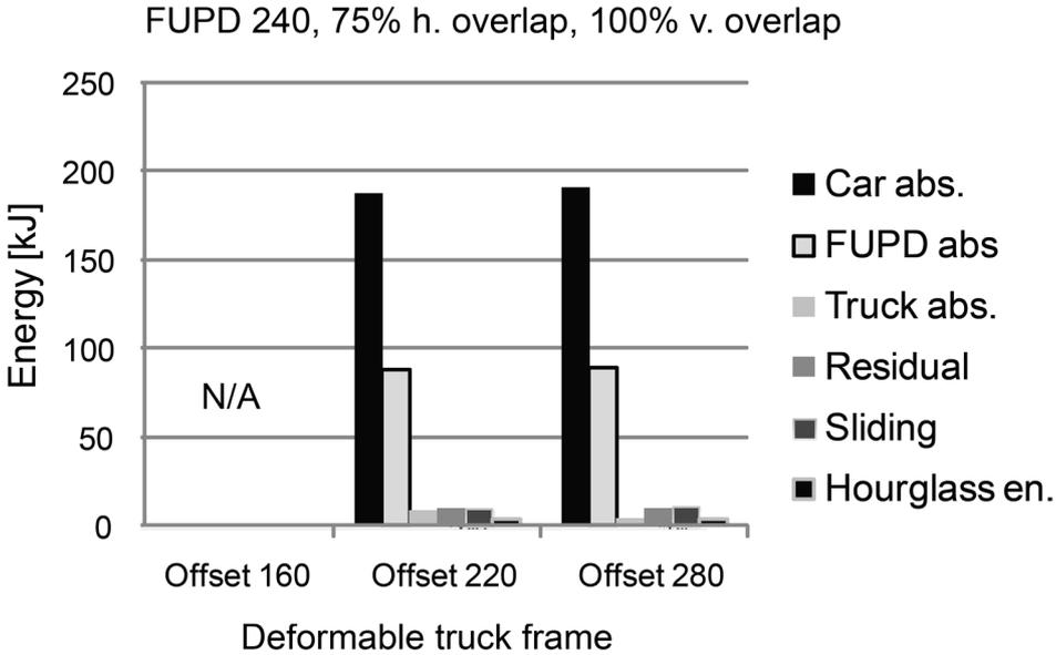
Figure 16: Comparison of energy distributions for different offsets for the FUPD of 240 mm cross-beam and deformable truck rails
