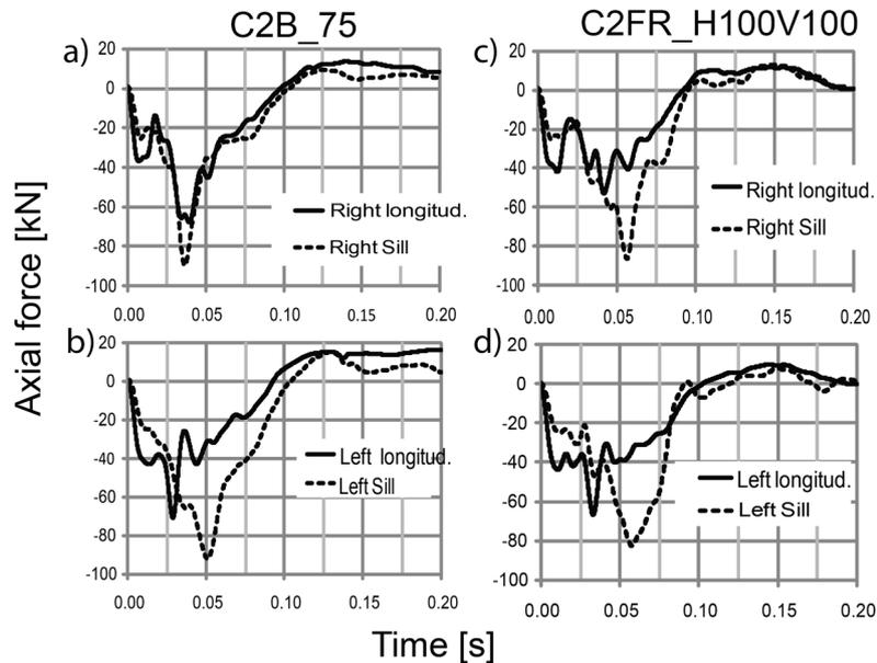
Figure 18: Axial loads measured in the right [(a) and (c)] and left [(b) and (d)] longitudinal structures of the car when crashed against FWRB [(a) and (b)] and against e.a. FUPD (c)
