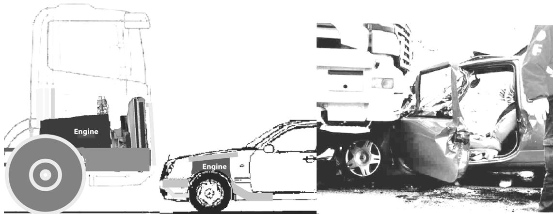
Figure 1: *Vertical misalignment between load paths of a passenger car and a truck (left) and its consequence (right)*
