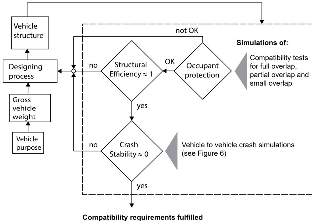
Figure 19: Implementation steps of the RED method on design process: Steps leading to compatibility
