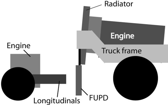
Figure 6: Proposed modification of front truck design
