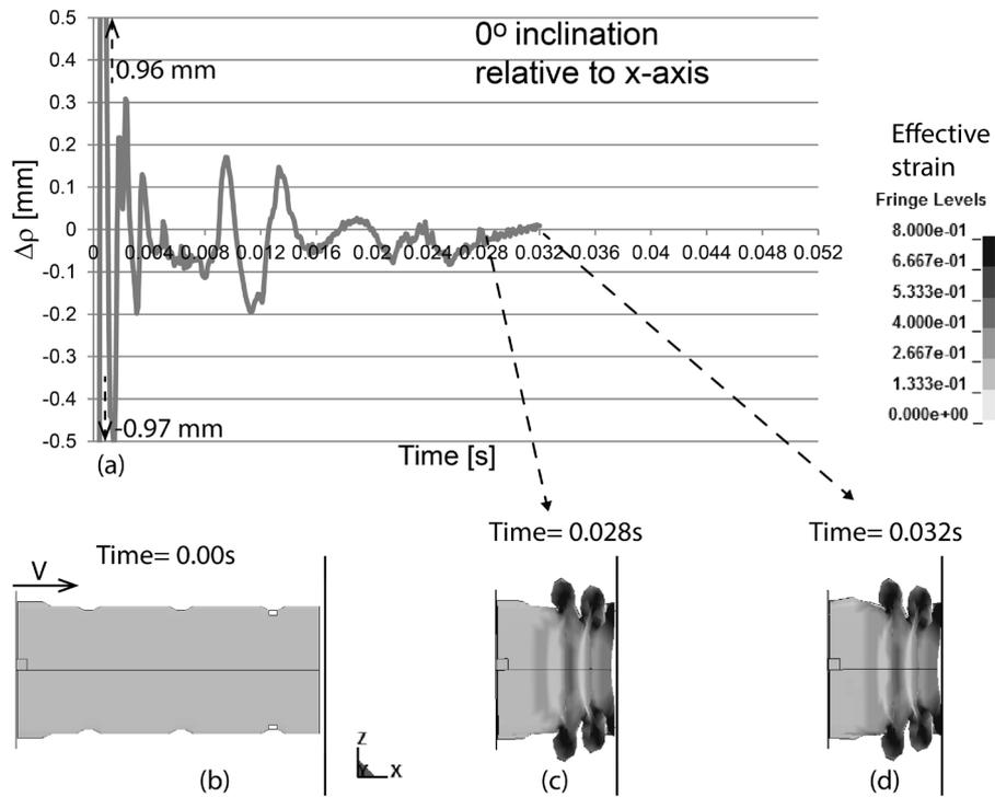
Figure 13: *Crash body 1 - 0° inclination relative to x-axis. (a) RED curve, (b) initial state just before impact, and states at approximate time points when (c) the buckling stops and (d) displacement reaches its maximum value, respectively at lower row with effective strain fringe pattern.*
