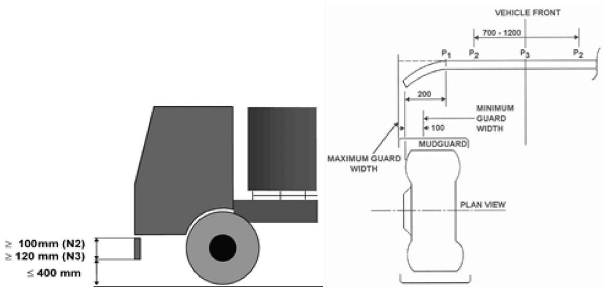
Figure 3: *Regulation 93 – Dimension limits and forces that FUPD has to sustained in the static component test.*
