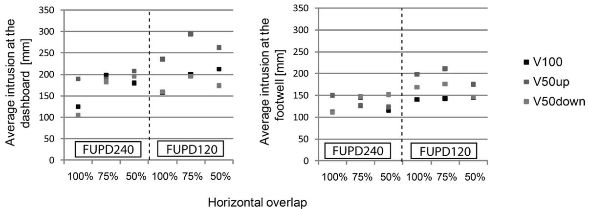
Figure 10: Average intrusions at firewall for different crash configurations in impact between the car and FUPD of two cross-beam sizes
