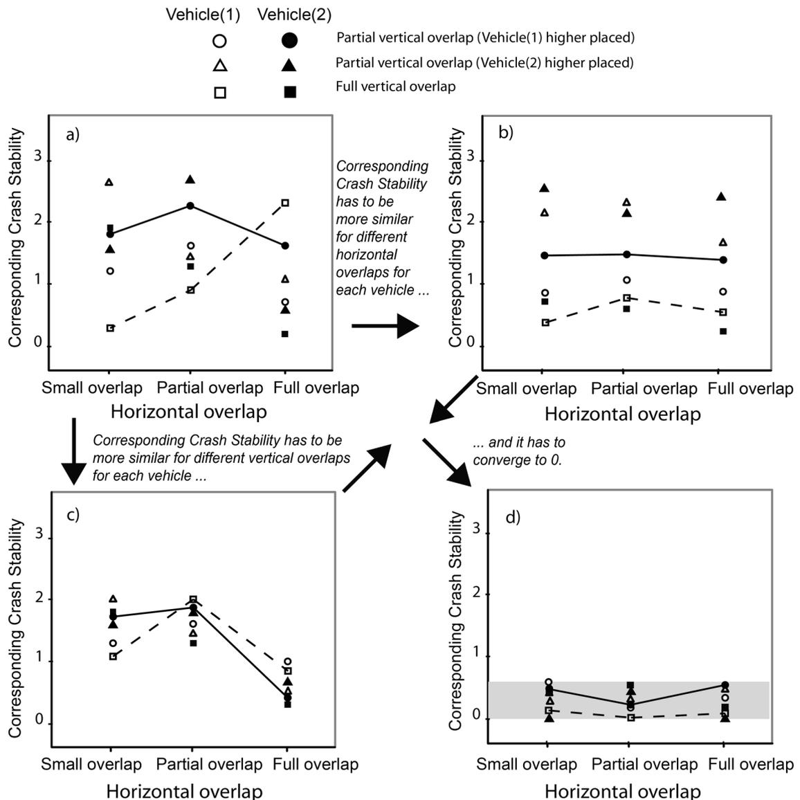
Figure 20: Steps leading to Crash Stability d) starting from a) imaginary results from car crash against itself simulations through b) prerequisites for achievement of compatibility performances in horizontal and c) vertical direction
