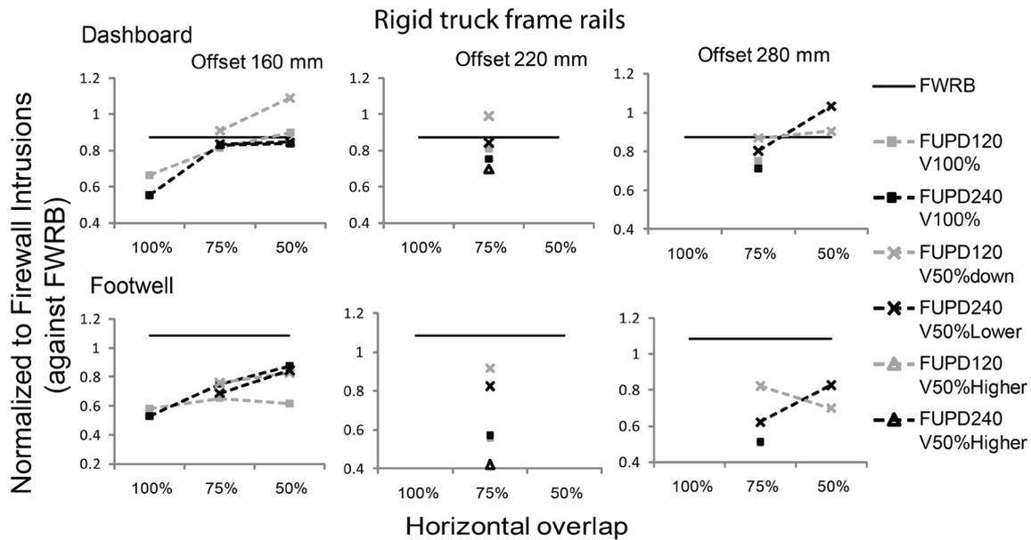
Figure 11: Calculated intrusions of the dashboard and footwell of the car impacting the truck with rigid frame rails
