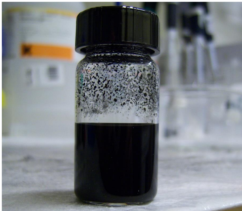
Figure 6. Carbon nanotube suspension using Triton X-100 as dispersion agent.
