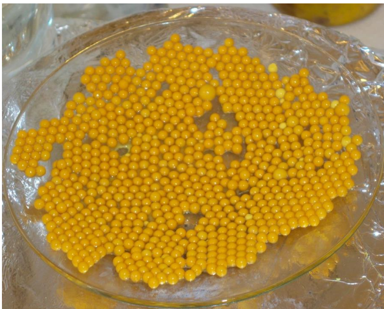
Figure 12. Gelled uranium microspheres produced by internal sol gel technique. Beads have been washed in petroleum ether and ammonium hydroxide and are left for drying.
