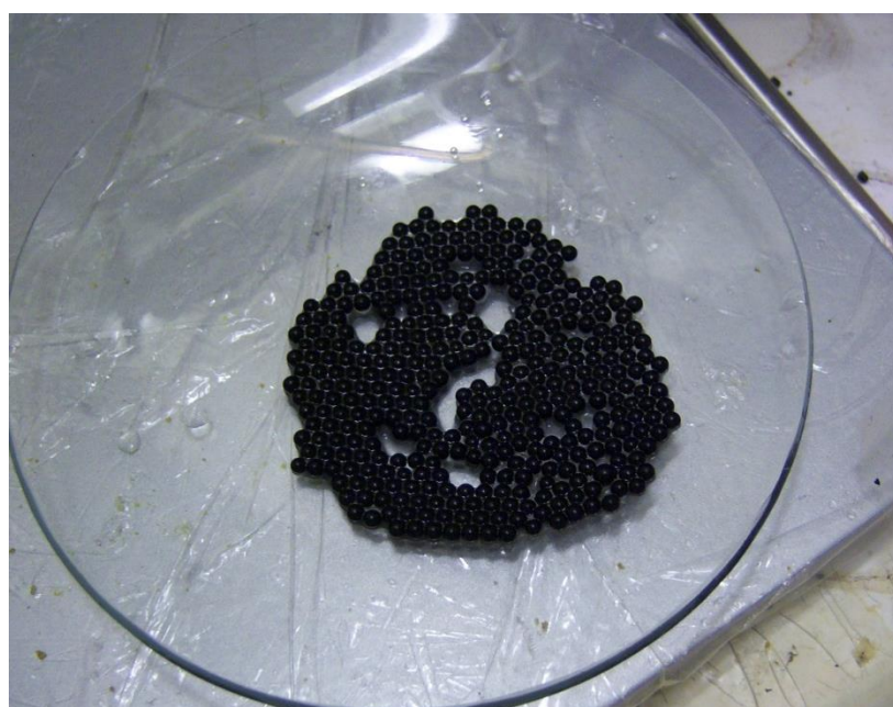
Figure 7. Picture of produced zirconium + CNT microspheres after washing in petroleum ether and aqueous ammonia and ageing in aqueous ammonia.
