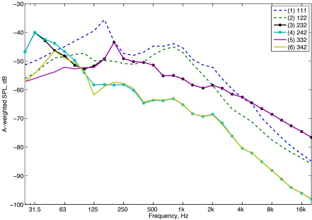
**Figure 4.** Calculated indoor noise levels for the suggested facade cases. The outdoor source strength is according to a frequency extended  $C_{tr}$  spectrum and the indoor level for each case is due to the combined transmission through wall, window and air intake. Key to the legend: first position is type of facade wall (1, 2 or 3), second position is type of window (1, 2, 3 or 4) and third position is type of air intake (1 or 2).
