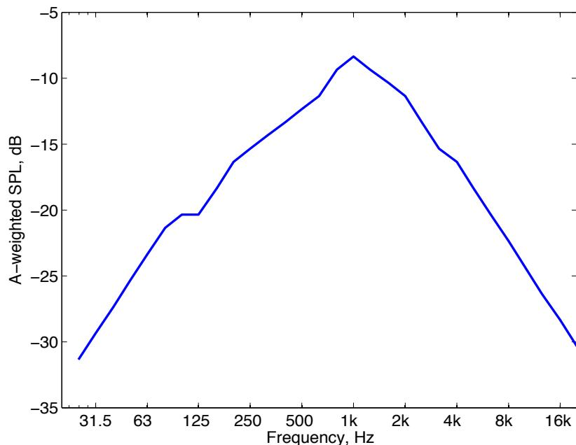
**Figure 1.**  $C_{tr}$  spectrum in the frequency extended version used here. Plotted is A-weighted sound pressure level, normalized to 0 dB(A).
