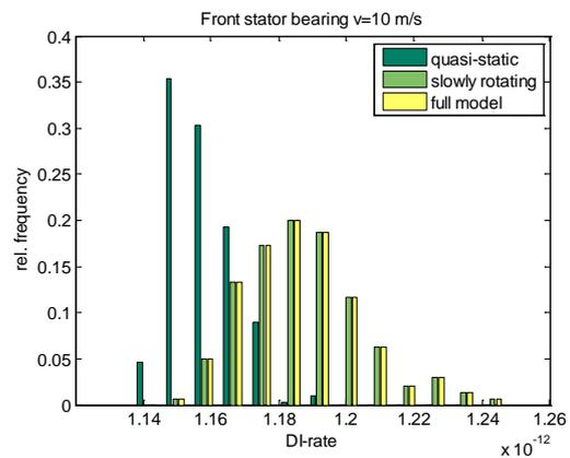
Figure 4: For front stator bearing, damage rate for mean wind speed 10 m/s, 300 realizations comparison of three drive train model details. The quasi-static model assumption strongly affects damage index rate distribution.
