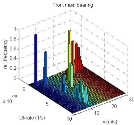
Figure 6: Histogram of damage index rate for front main bearing at different mean wind speeds.
