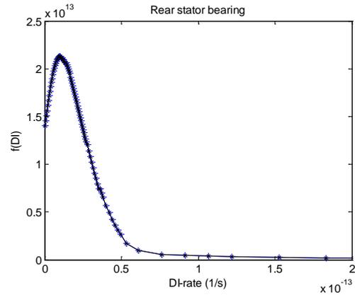
Figure 13: Distribution of total damage rate for rear stator bearing.
