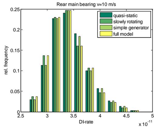
Figure 3: For rear main bearing, damage rate for mean wind speed 10 m/s, 300 realizations comparison of four drive train model details. Damage index rate distribution appears independent of model.
