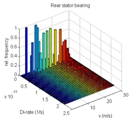
Figure 9: Histogram of damage index rate for rear stator bearing at different mean wind speeds.
