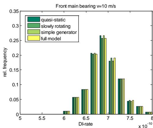
Figure 2: For front main bearing, damage rate (Eqn. 1) for mean wind speed 10 m/s, 300 realizations comparison of four drive train model details. Damage index rate distribution appears independent of model.
