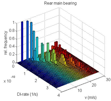
Figure 7: Histogram of damage index rate for rear main bearing at different mean wind speeds.
