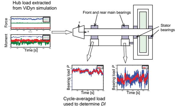
Figure 1: Drive train simulation setup.
