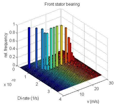
Figure 8: Histogram of damage index rate for front stator bearing at different mean wind speeds.
