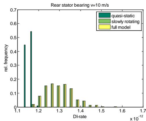
Figure 5: For rear stator bearing, damage rate for mean wind speed 10 m/s, 300 realizations comparison of three drive train model details.
