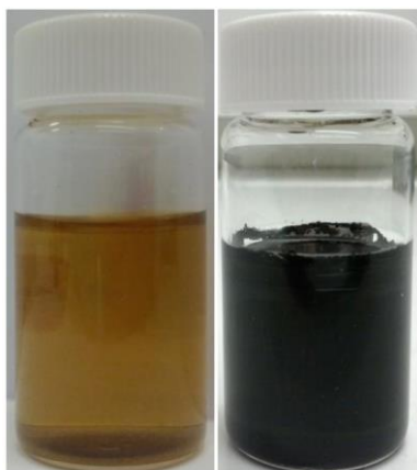
Figure 4.2 Typical appearance of the aqueous (left) and oil phases (right) after centrifugation.
