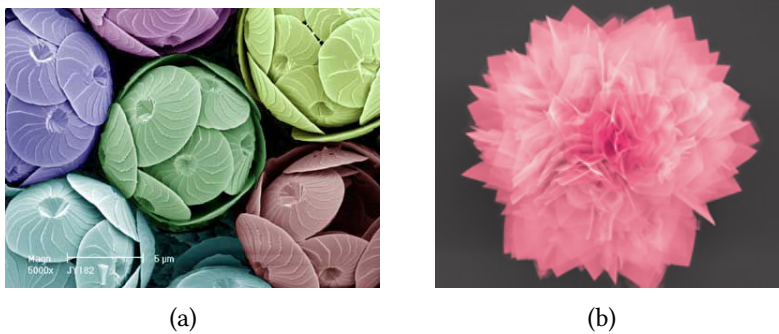
Figure 1.1: (a) Calcidiscus, a biomineralized crystalline product (from the International Nanoplankton Association website). (b) Nano-Flower, a germanium-sulfide nanosheet structure (from the Materials Research Society).
