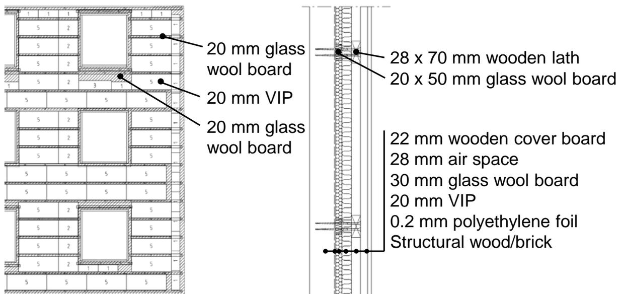
Figure 4.3. Wall layout after retrofitting with 20 mm VIP and 30 mm glass wool boards. (Figure 5 in Paper IV).
