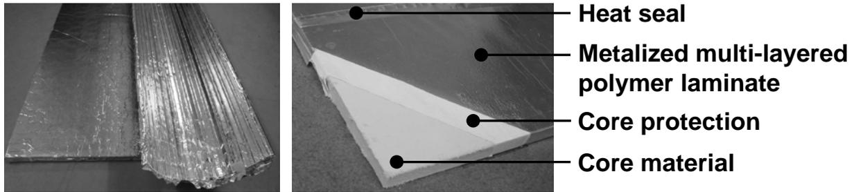
Figure 2.5. Left: flat and concave VIP for use as pipe insulation (Photo: Axel Berge). Right: the fine powder core is wrapped in a heat sealed metalized multi-layered polymer laminate (Photo: va-Q-tec AG).
