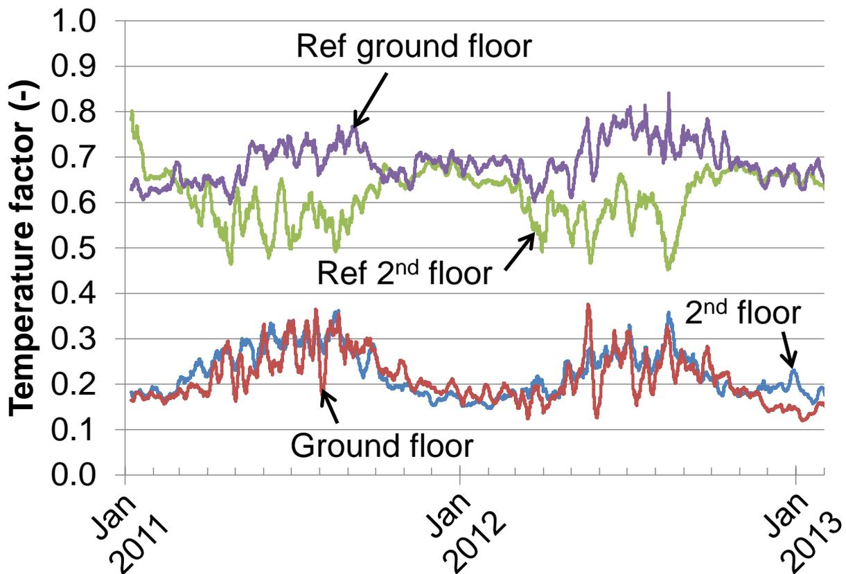
Figure 4.7. Weekly averaged temperature factor over the part of the wall on the interior of the sensor during 2011, 2012 and January 2013.
