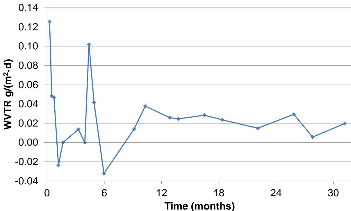
Figure 2.8. Measured average WVTR of six samples of a metalized triple-layered polymer laminate by the wet cup method in  $23^\circ\text{C}$  and 50% RH stored in the laboratory at Chalmers. The weight was determined on a scale with 0.01 g resolution.
