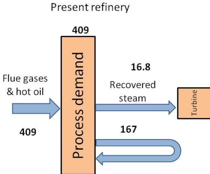
Figure 1 Heat balance of the present refinery
