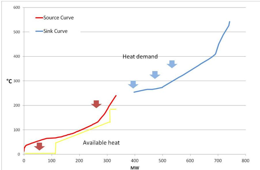
Figure 11 Process source and sink curve showing available heat and heat demand. The cold utility line show today's utility with possible surplus steam generation and heat cooled with air or cooling water. The heat demand is covered with flue gases from furnaces.
