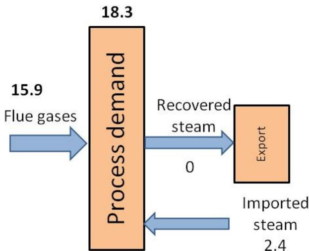
Figure 3 Heat balance of the present unit SynSat
