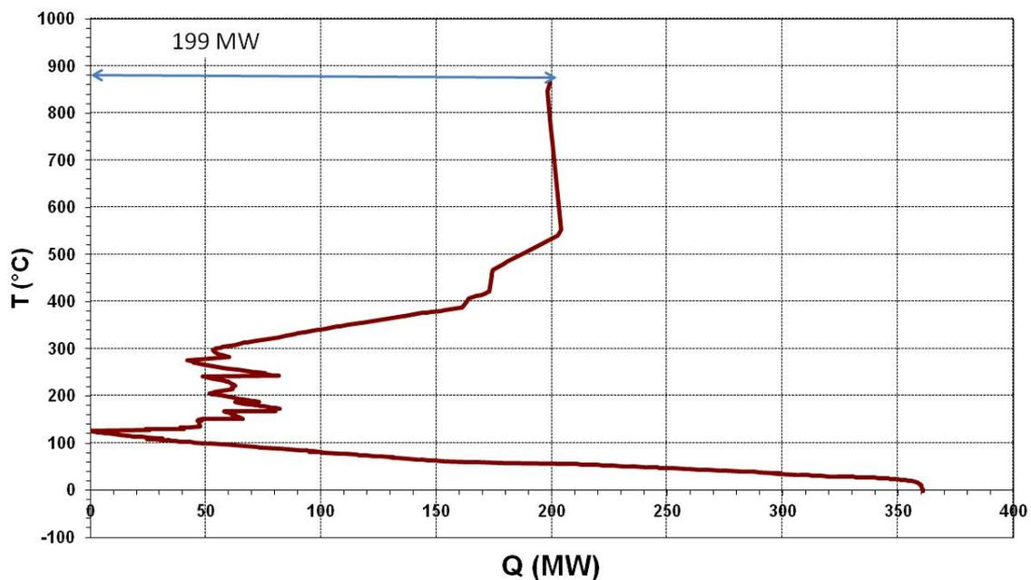
Figure 7 Grand Composite Curve including all streams at the refinery. The figure show that the minimum heat demand,  $Q_{h, min}$  is 199 MW.
