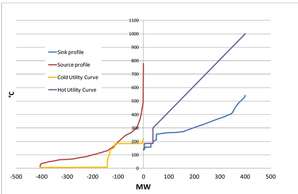
Figure 6 The Source Profile (hot process streams) that are cooled with cold utility (Cold Utility Curve) – the and the Sink Profile (cold process streams) that are heated with hot utility (Hot Utility Curve)
