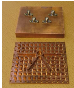
Figure 5. 11 Photo of the 15 – 17.5 GHz 3dB hybrid in ridge gap waveguide. The texture plate showing the ring hybrid surrounded by metal pins.
