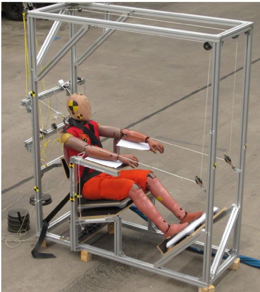
Figure 3-1: Test rig when used to evaluate shoulder range-of-motion of a THORAX dummy.
