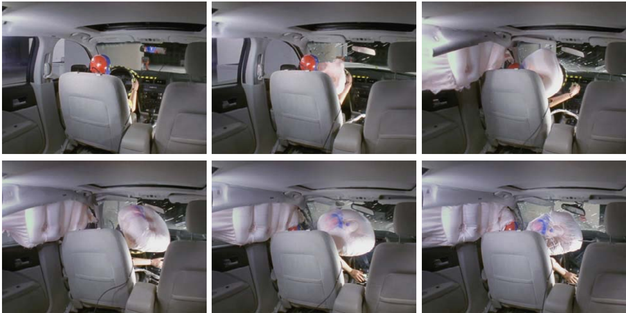
Fig 3. 5 th percentile female Hybrid III dummy kinematics in IIHS test CF11012 with a 2008 Ford Fusion.
