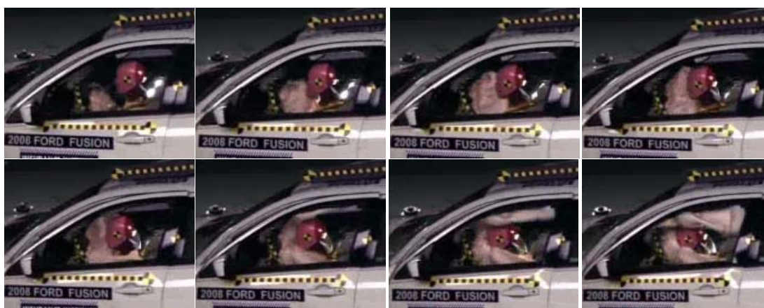
Fig 7. 5 th percentile female Hybrid III dummy neck and airbag interaction in IIHS test (CF11012).
