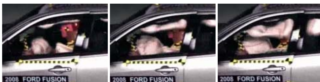
Fig 8. 50 th percentile male Hybrid III dummy neck and airbag interaction in IIHS test (CF11002).
