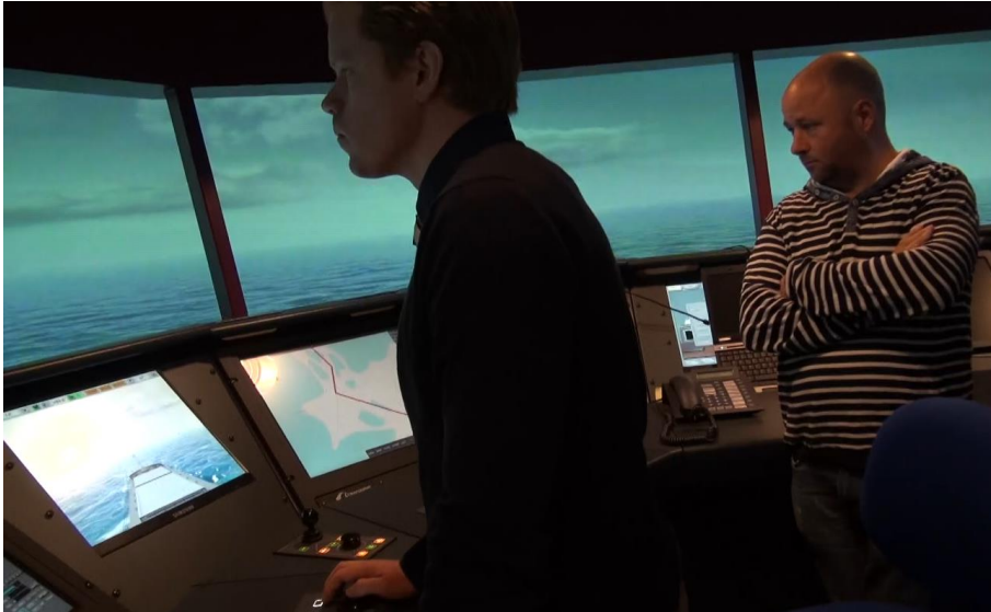
Figure 4. Watch officer and captain on the simulator bridge. The route is visible in the prototype screen (scenario 4, before the MSI with drifting timber has been received).
