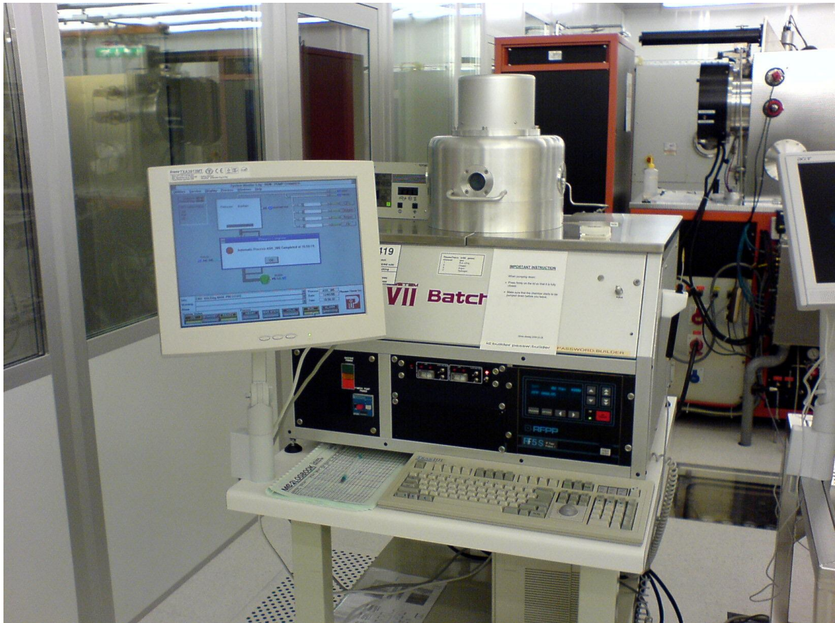
Figure 6.3: The Plasma Therm Batchtop PE/RIE m/95 used for etching.
