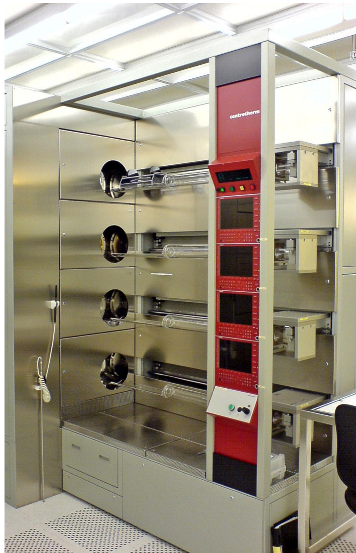
Figure 5.1: The Centrotherm LPCVD horizontal furnace.
