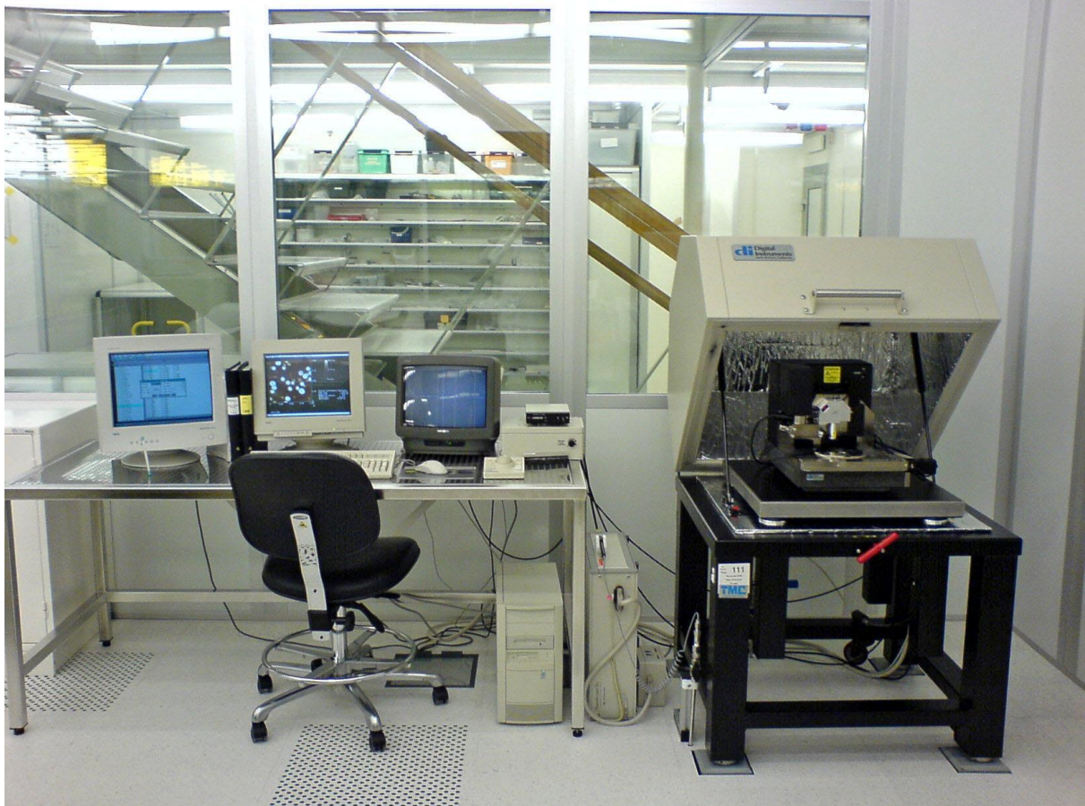
Figure 6.2: The Digital Instrument Dimension 3000 SPM used for roughness measurements.
