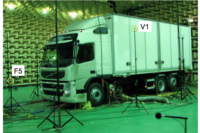
Figure 1: The sound of the Volvo FM truck was recorded in a semi-anechoic laboratory. Microphone positions F5 and V1 are indicated by circles.
