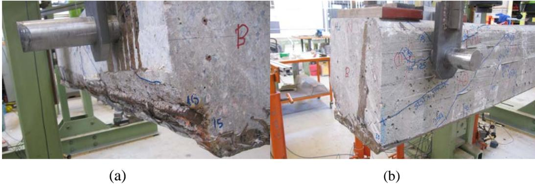
**Figure 7.** (a) Spalling along the main bundled bars 15 and 16 in beam H7. (b) Splitting-induced crack failure on the front-side in beam H7.
