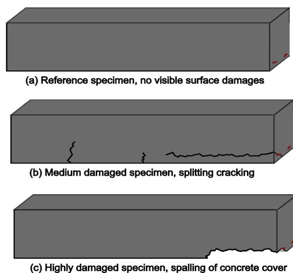
**Figure 4.** Categorization of the specimens based on different extents of corrosion induced
