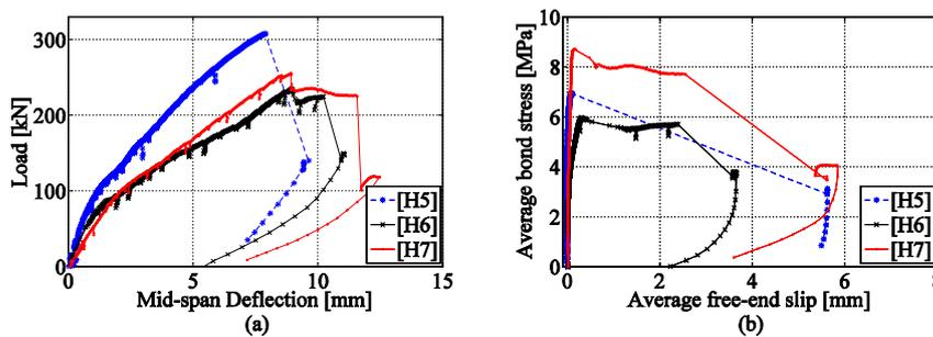
**Figure 10.** (a) Average load in the hydraulic jacks versus deflection at mid-span. (b) Average bond stress versus the average free-end slip for the Highly damaged specimens.
