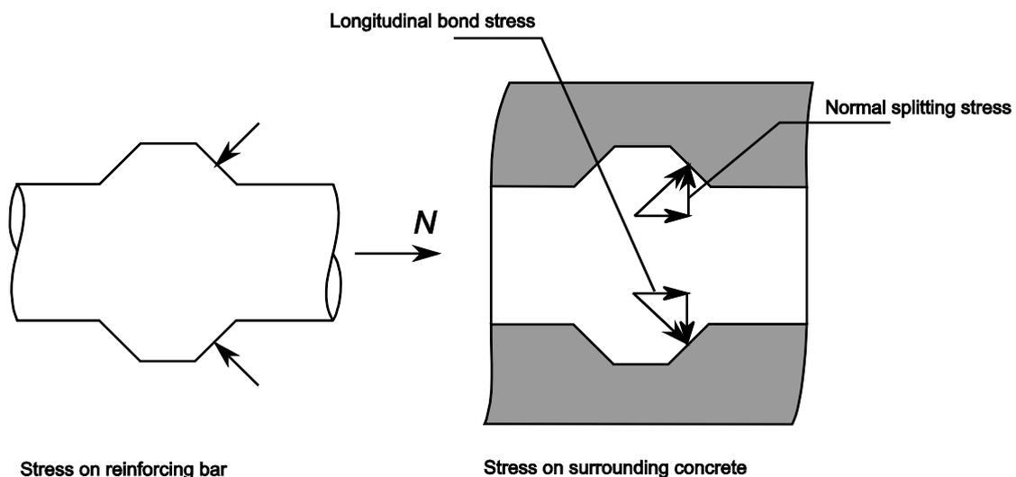
**Figure 3.** Bond between a ribbed bar and the surrounding concrete by mechanical interlocking, as modified from Magnusson (2000).
