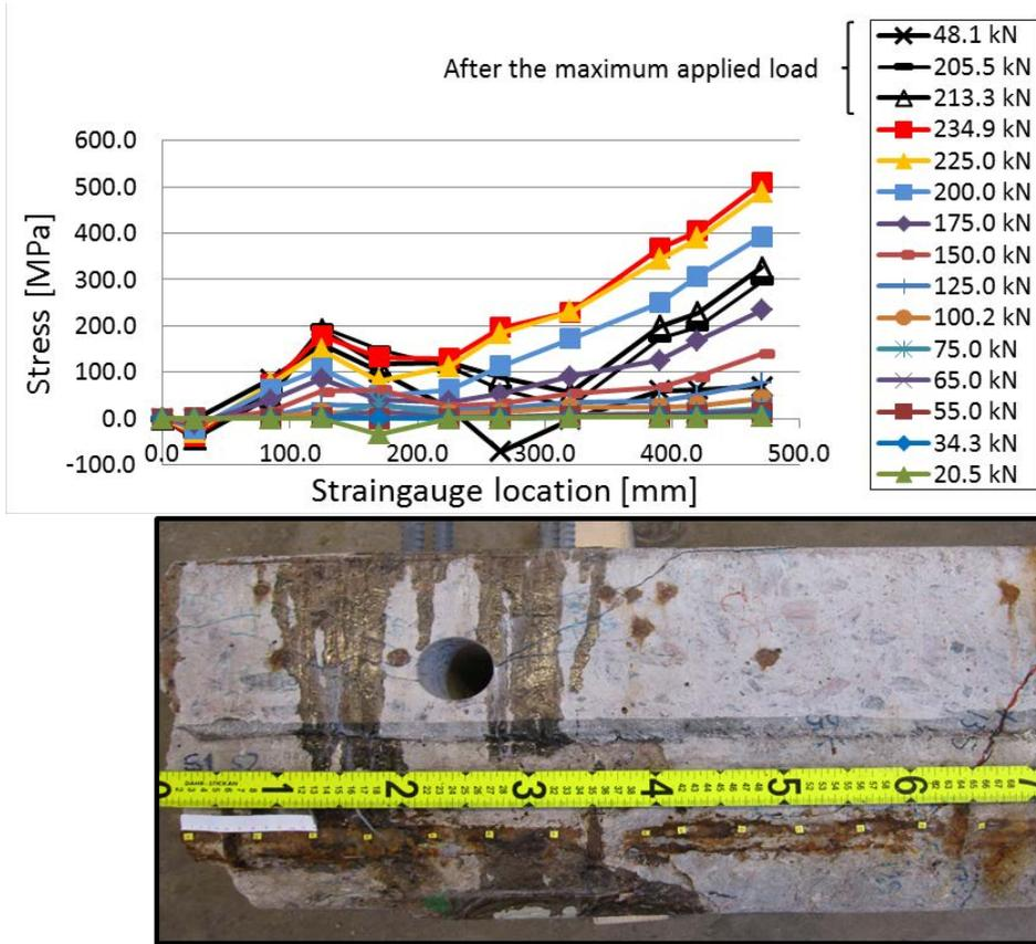
**Figure 8.** Measured strains on a longitudinal bar in specimen (H6) and the distribution of stresses in different load increments in the anchorage zone.
