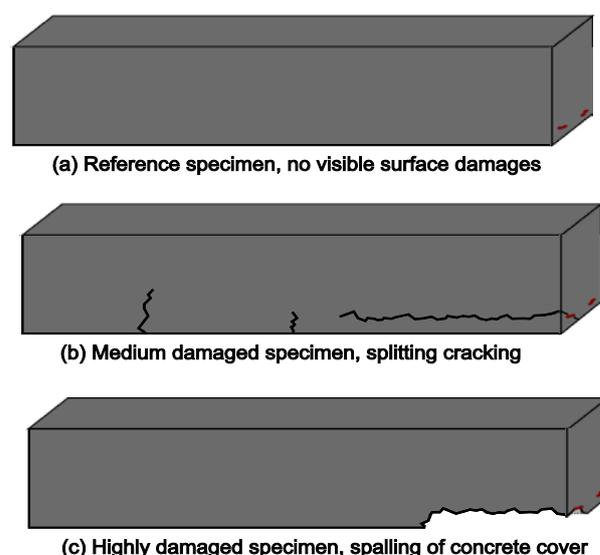
**Figure 4.** Categorization of the specimens based on different extents of corrosion induced
