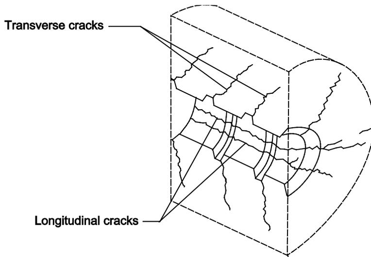
**Figure 2.** Longitudinal and transverse cracks caused by bond, as modified by Magnusson (2000) from Vanderwalle (1992).
