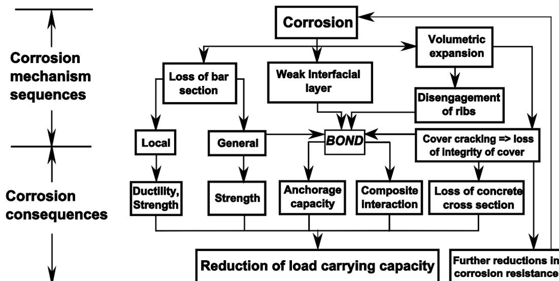
Figure 1. Mechanism sequences and consequences of corrosion on reinforcements, reproduced from (Cairns et al., 1999).
