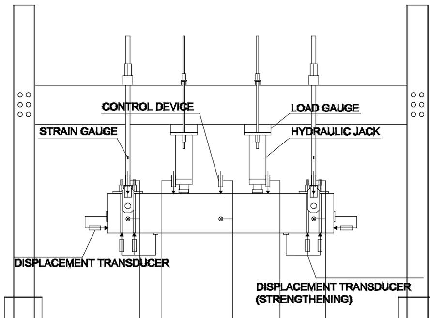
**Figure 5.** Four-point bending test with indirect supports.
