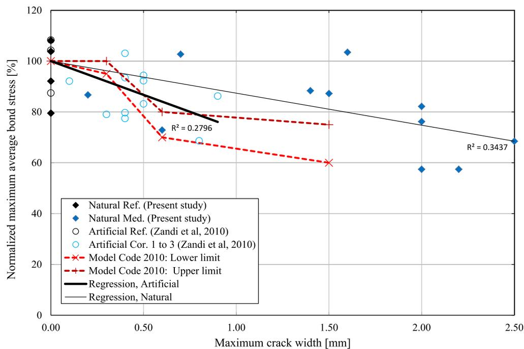
**Figure 11.** Comparison of test results from the naturally corroded specimens with artificially corroded tests and with Model Code 2010 in terms of bond strength, normalized with respect to the average maximum bond strength obtained from reference samples, versus maximum crack width of splitting cracks.
