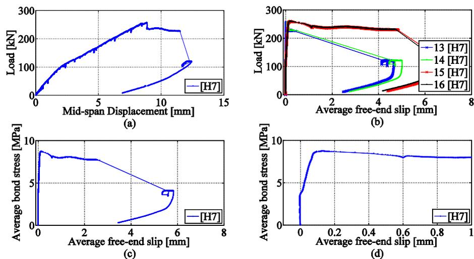
**Figure 6.** Overview of results from test H7: (a) Average load in the hydraulic jacks versus deflection at mid-span; (b) Average load from the hydraulic jacks versus the end slips in each of the bundled bars; (c) Average bond stress versus average free-end slip; (d) Enlarged figure of (c).
