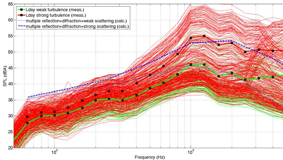
Figure 4 – Measured and calculated spectra at the shielded location. All hourly equivalent sound pressure level spectra are shown as well (thin green and red lines) that form the basis for the energetically averaged values  $L_{day}$ .
