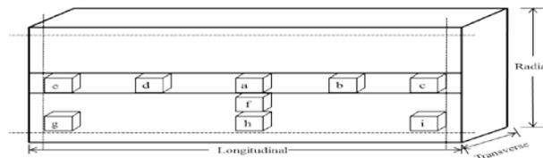
Figure 1. Different cubical portions from 100x50x4 mm chip used in the concentration profile measurements.
