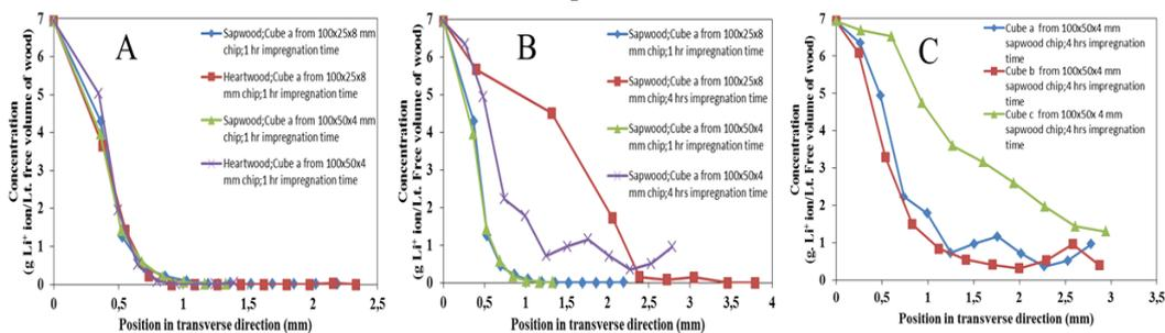
Figure 2. Measured concentration profiles of  $\text{Li}^+$  ion in Norway spruce wood chips at room temperature: A. Sapwood vs. Heartwood, 1 hr impregnation time; B. 1 hr vs. 4 hrs impregnation time, Sapwood; C. At various locations within a single wood chip.
